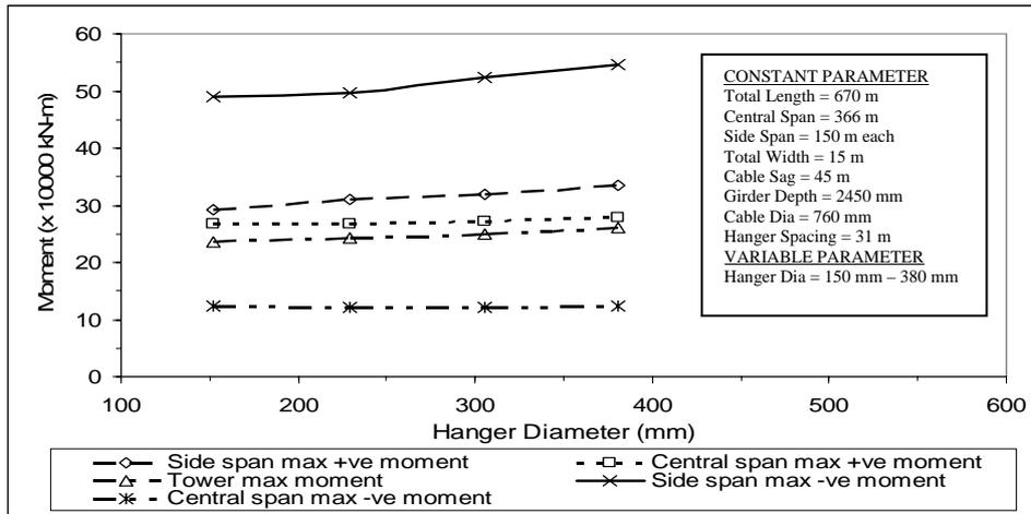
Fig. 14. Variation of maximum tower, central and side span maximum moments with hanger diameter
