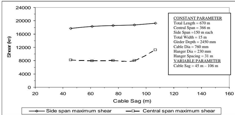
Fig. 4. Variation of central and side span maximum shear with cable sag
