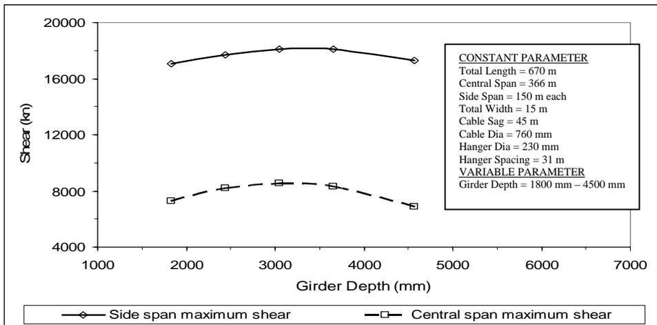
Fig. 8. Variation of central and side span maximum shear with girder depth
