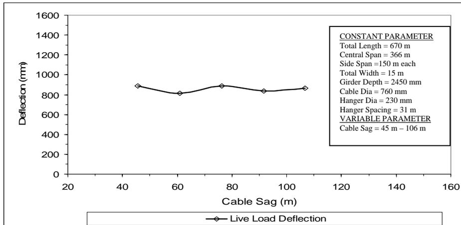
Fig. 5. Variation of maximum live load deflection with cable sag
