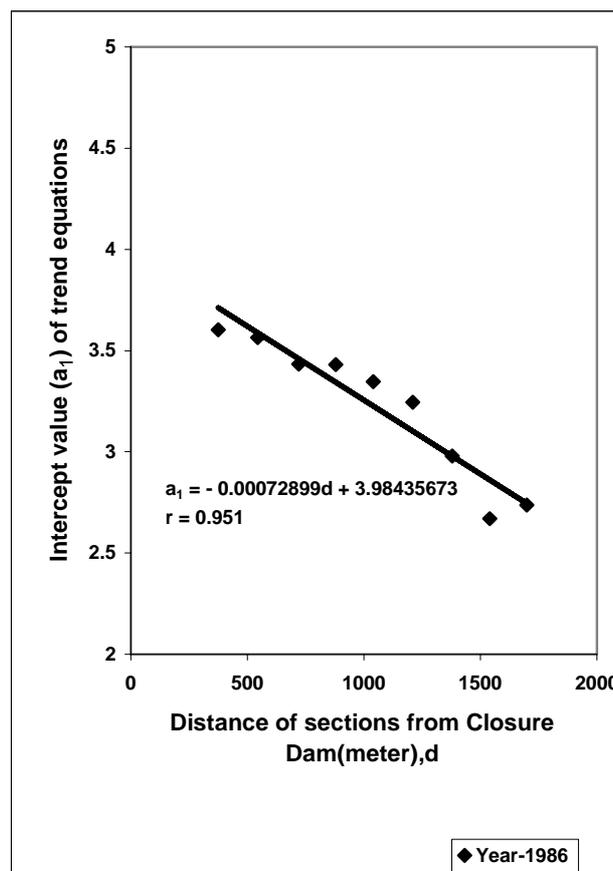
Fig. 2. Relation between intercept values of accretion height equations and the closure distance
