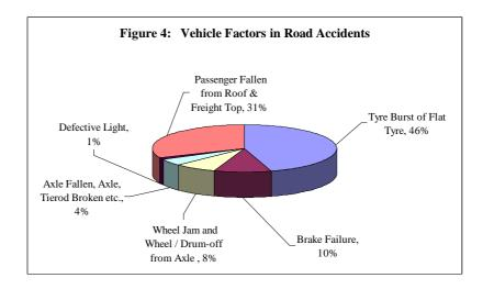
Figure 4 shows that tyre bursts constituted about 46% of the pie followed by passenger fall down (31%), defective brakes (10%), defective wheels (8%), axle and tierod fault (4%), and defective light (1%).
