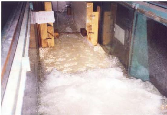
Fig. 9. Jump is approaching towards the expansion section due to raising the tail water gate.
