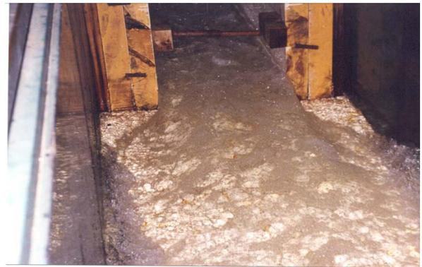
Fig. 10. Initial stage of jump formation in an expanding channel
