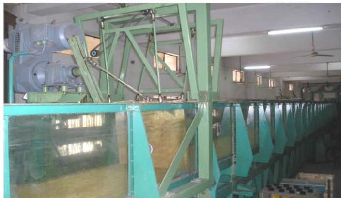
Fig. 3. 21.3 m long laboratory flume for the research
