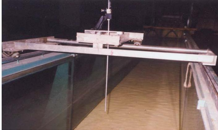
Fig. 6. Photograph of point gauge
