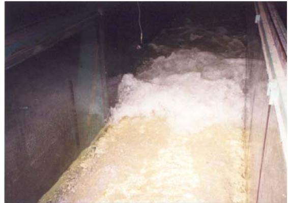
Fig. 8. Hydraulic jump in a horizontal rectangular channel.
