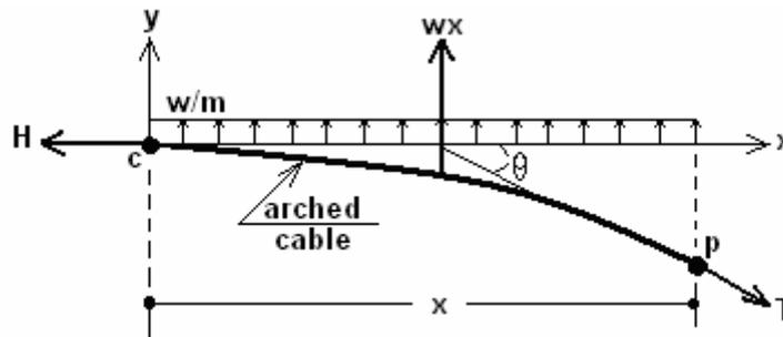
Fig.4 The forces acting on a portion of an arched cable.
