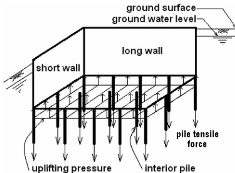
**Fig.1- A bottom isometric view of a rectangular underground tank subjected to an uplifting pressure.**
