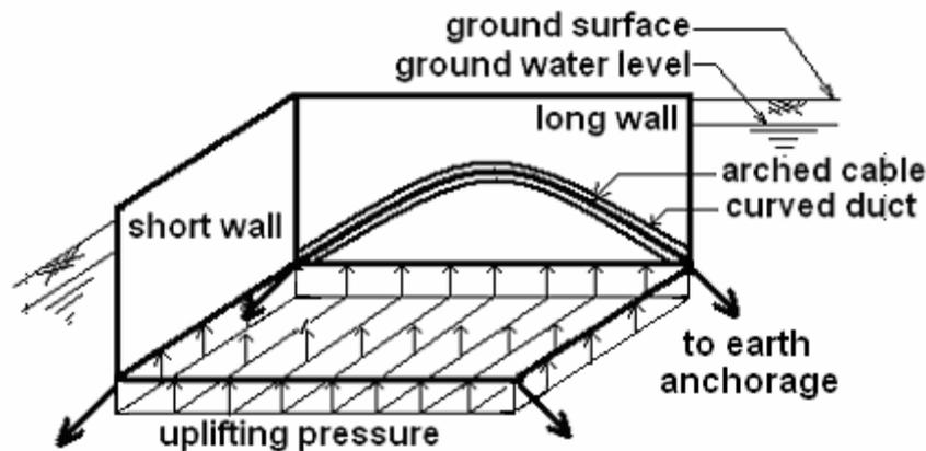
**Fig.2- A typical rectangular underground tank stabilized by two arched cables.**
