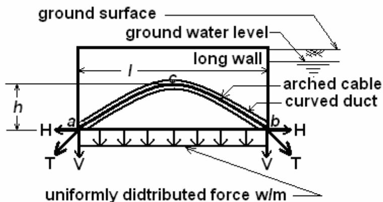
Fig.3-Type of loading exerted by an arched cable.
