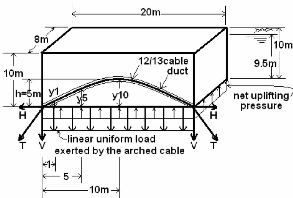
**Fig.5- A rectangular reinforced concrete underground tank, stabilized against flotation by two arched cables.**
