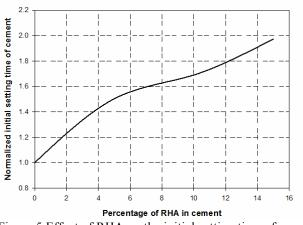
Figure 5 Effect of RHA on the initial setting time of cement
