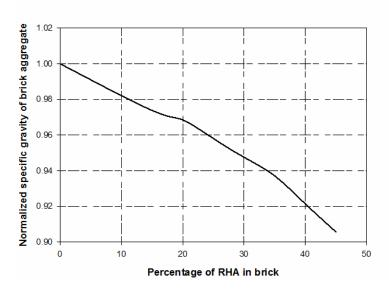
Figure 13. Effect of RHA on the specific gravity of brick aggregate
