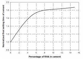
Figure 6. Effect of RHA on the final setting time of cement
