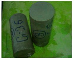
(a) Cylinder with partial replaced of cement with RHA
