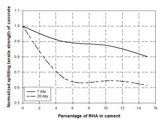
Figure 9. Effect of RHA on the splitting tensile strength of concrete
