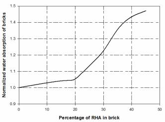
Figure 11 Effect of RHA on the water absorption of bricks.
