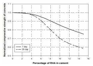
Figure 8. Effect of RHA on the compressive strength of concrete
