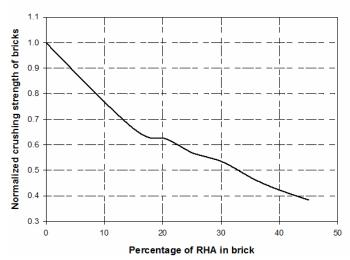
Figure 12. Effect of RHA on the crushing strength of bricks
