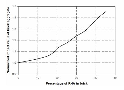
Figure 14. Effect of RHA on the impact value of brick aggregate
