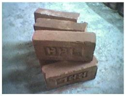
(b) Brick with partial replaced of clay with RHA
