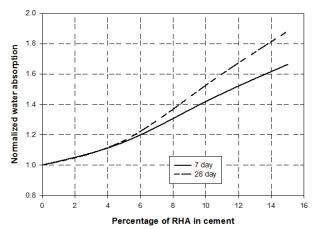
Figure 7. Effect of RHA on the water absorption of concrete
