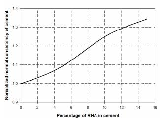
Figure 4 Effect of RHA on the normal consistency of cement
