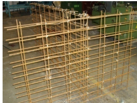
Fig. 5. BRC detailing of wall-slab
