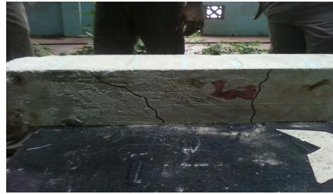
(b) Shear failure of RCC beam
