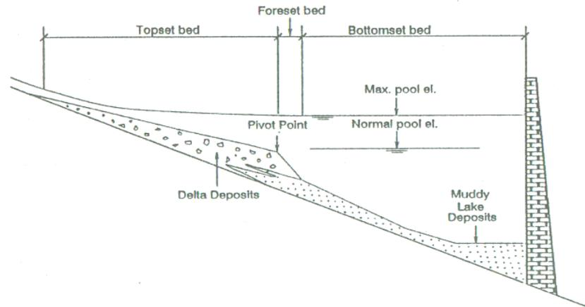
Fig. 1. Longitudinal profile of delta sedimentation in reservoir (Morris and Fan, 1998)
