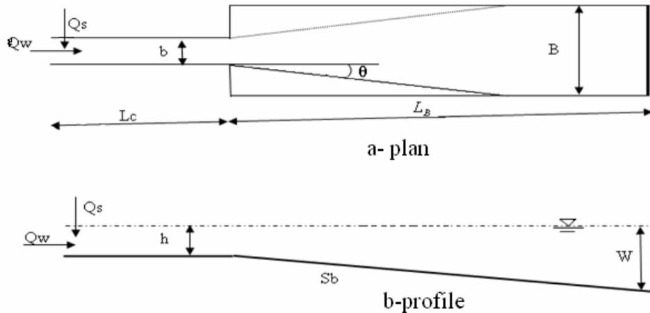
Fig. 2. Plan and longitudinal profile laboratory flume
