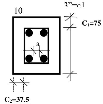
$$c_1 = 75 \text{ mm (top covering)}, \quad c_2 = 37.5 + 10 + \frac{36}{2} = 65.5 \text{ (mm)}$$
