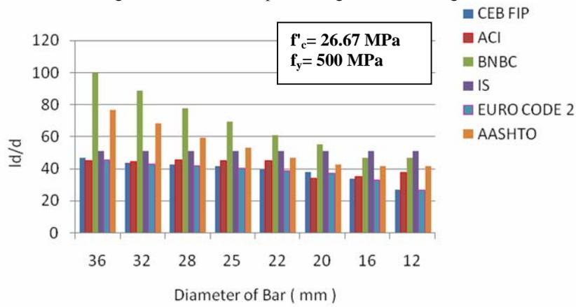
Fig. 25. Tension development length of reinforcing bar.
