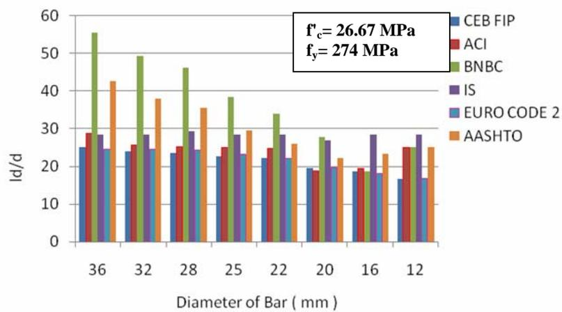
Fig. 11. Tension development length of reinforcing bar.
