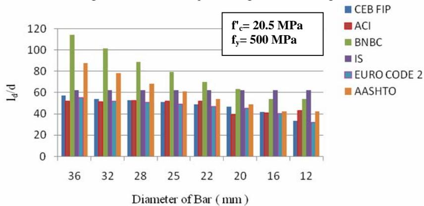
Fig. 23. Tension development length of reinforcing bar.
