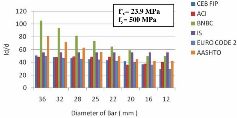
Fig. 24. Tension development length of reinforcing bar.
