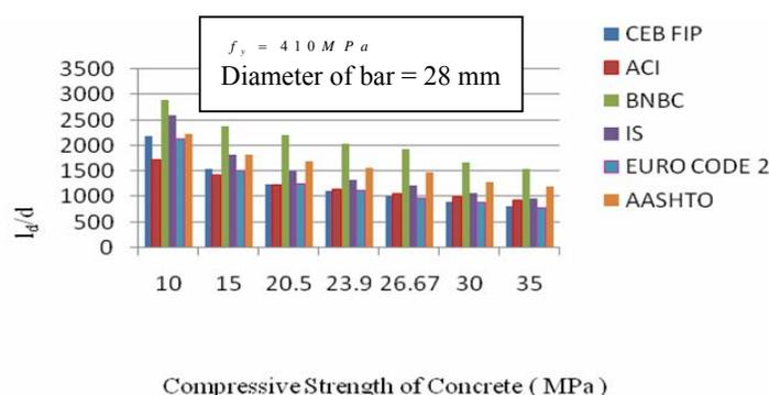
Fig. 30. Tension development length of reinforcing bar
