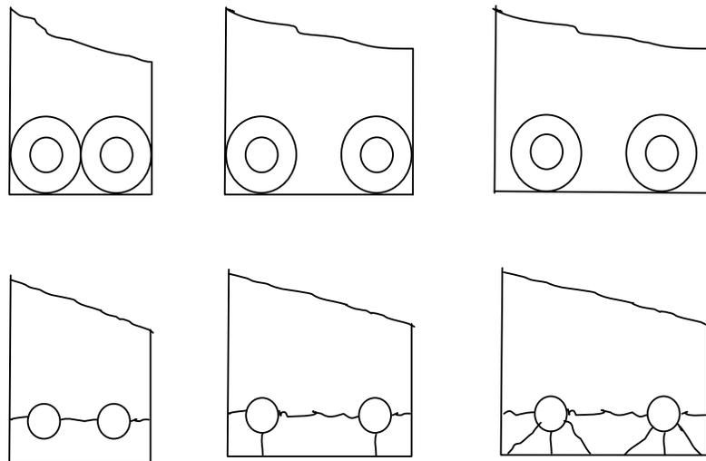
(a) Side cover and half the bar spacing both less than bottom cover.
