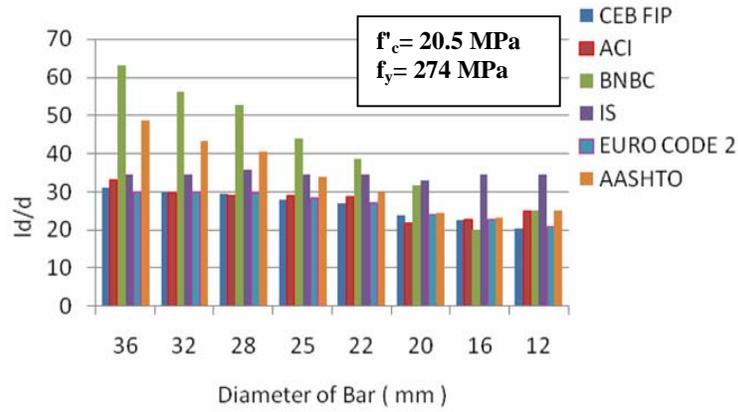
Fig. 9. Tension development length of reinforcing bar.
