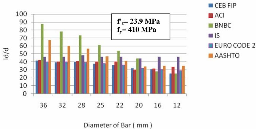
Fig. 17. Tension development length of reinforcing bar.
