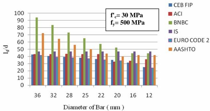
Fig. 26. Tension development length of reinforcing bar.
