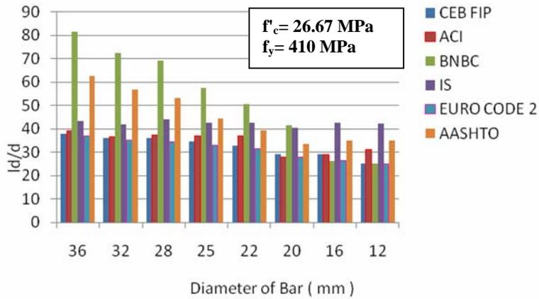
Fig. 18. Tension development length of reinforcing bar.
