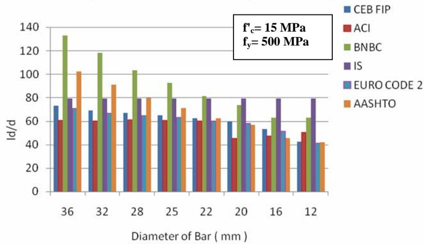
Fig. 22. Tension development length of reinforcing bar.
