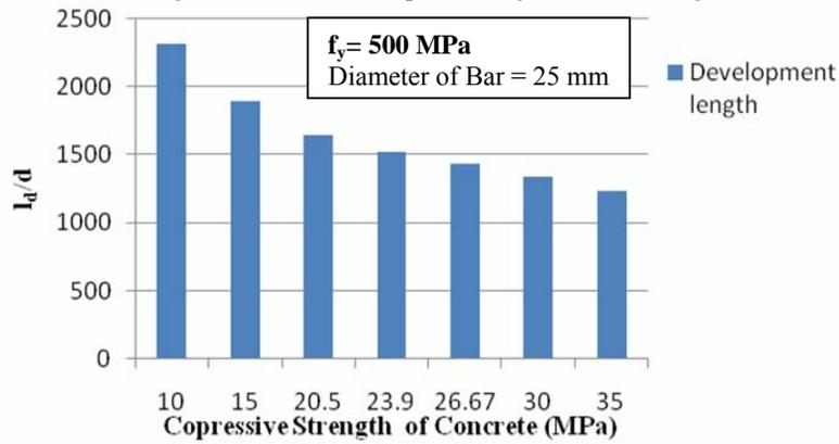
Fig. 28. Tension development length of reinforcing bar
