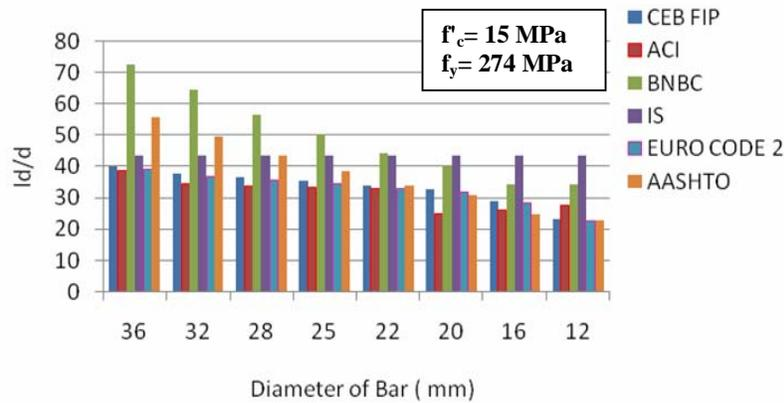
Fig. 8. Tension development length of reinforcing bar
