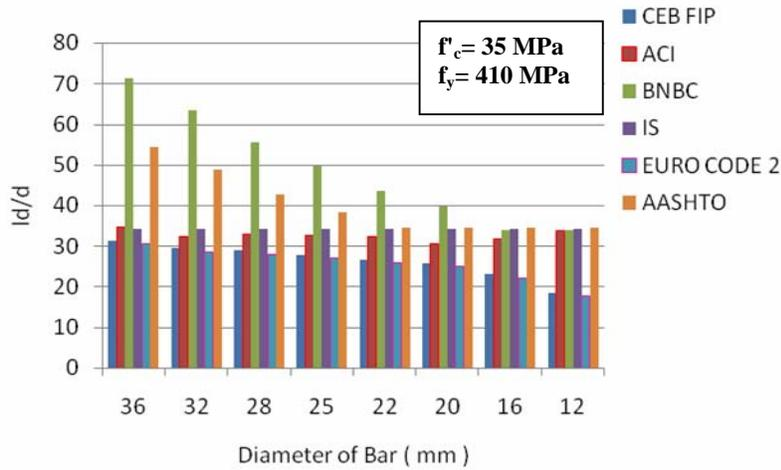
Fig. 20. Tension development length of reinforcing bar.
