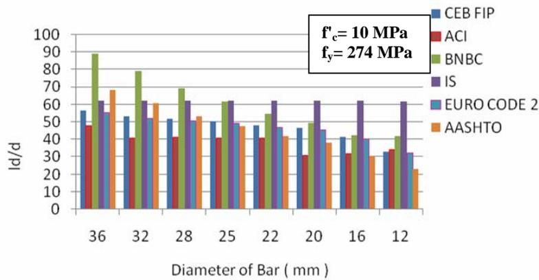
Fig. 7. Tension development length of reinforcing bar
