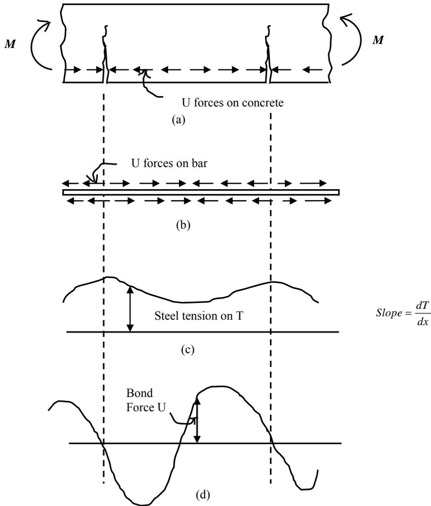
Fig. 1. (a) Cracked concrete segment, (b) bond stress acting on reinforcing bar, (c) variation of tensile force in reinforcing bar; and (d) variation of bond force along the bar (adapted from Nilson et al., 2005)
