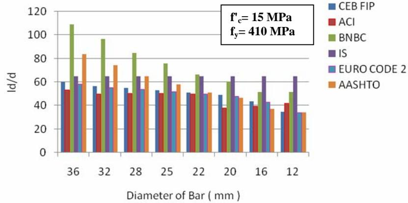
Fig. 15. Tension development length of reinforcing bar.
