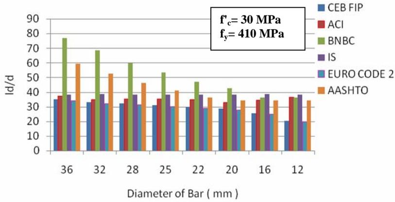
Fig. 19. Tension development length of reinforcing bar.
