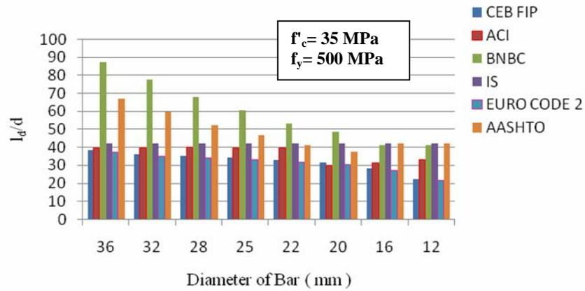
Fig. 27. Tension development length of reinforcing bar.
