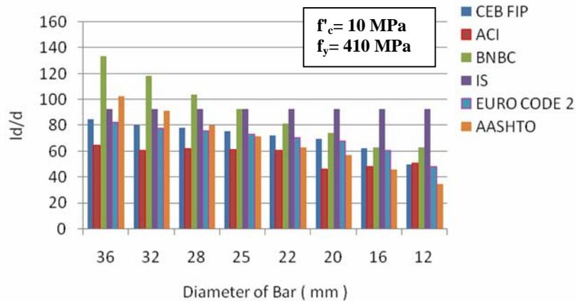
Fig. 14. Tension development length of reinforcing bar.
