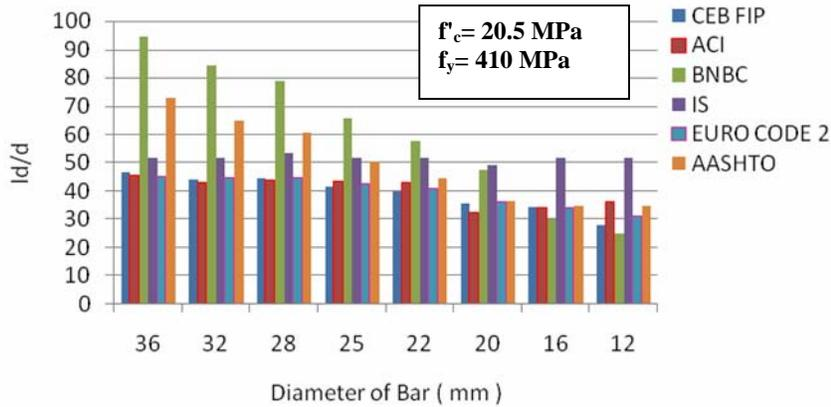
Fig. 16. Tension development length of reinforcing bar.
