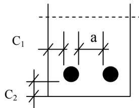
Fig.5.  $c_{min} = \min(a / 2, c_1, c_2)$
