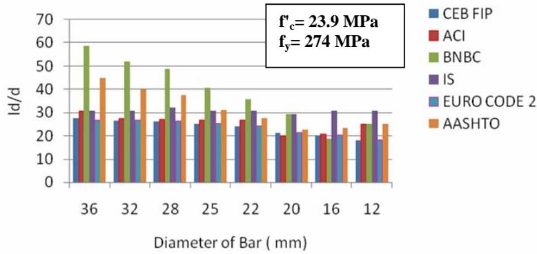
Fig. 10. Tension development length of reinforcing bar.
