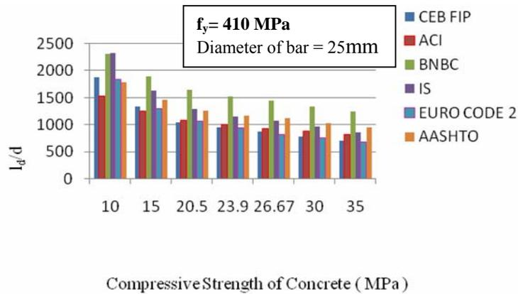
Fig. 29. Tension development length of reinforcing bar
