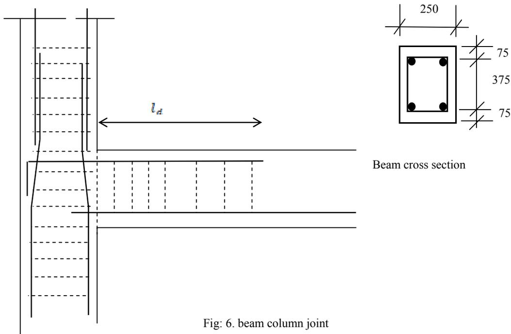
Fig. 6. beam column joint
