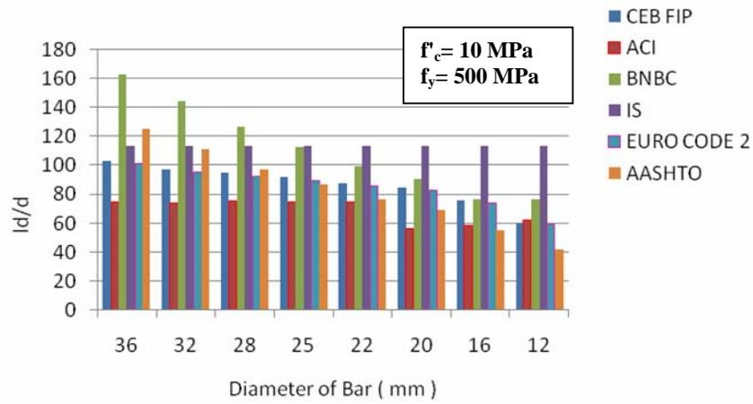
Fig. 21. Tension development length of reinforcing bar.
