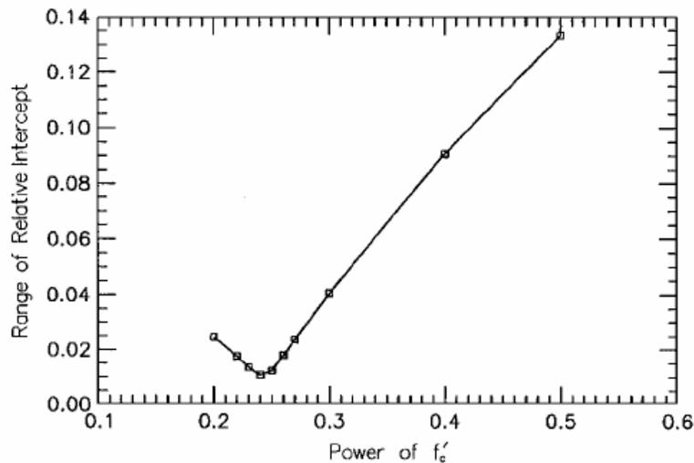
Fig. 4. Range of relative intercept obtained for dummy variables analysis for experimental bond force, normalized with respect to  $f'_c$  for optimized bond strength expressions versus the power  $p$  of  $f'_c$  for bars without confining transverse reinforcement. (Ref. David Darwin, 2005).
