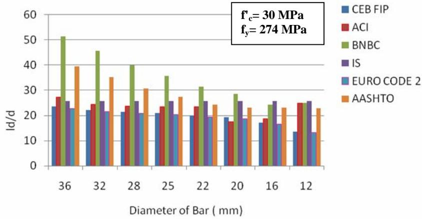
Fig. 12. Tension development length of reinforcing bar.
