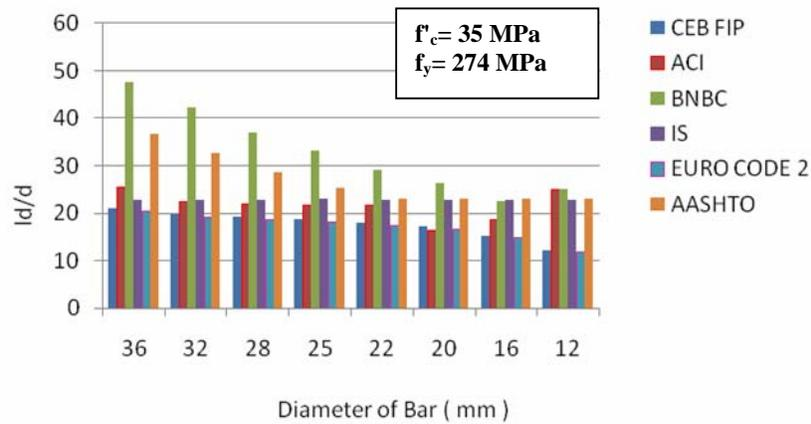
Fig. 13. Tension development length of reinforcing bar.
