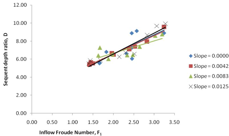
Fig. 4. D vs  $F_1$  graph for different channel slopes with drop height,  $\Delta z = 6$  cm
