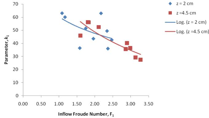
Fig. 5. Variation of parameter  $k_1$  with  $F_1$  for different drop height with Slope = 0.0042
