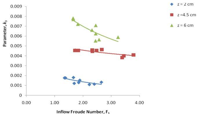
Fig. 7. Variation of parameter  $k_3$  with  $F_1$  for different drop height with Slope = 0.0042
