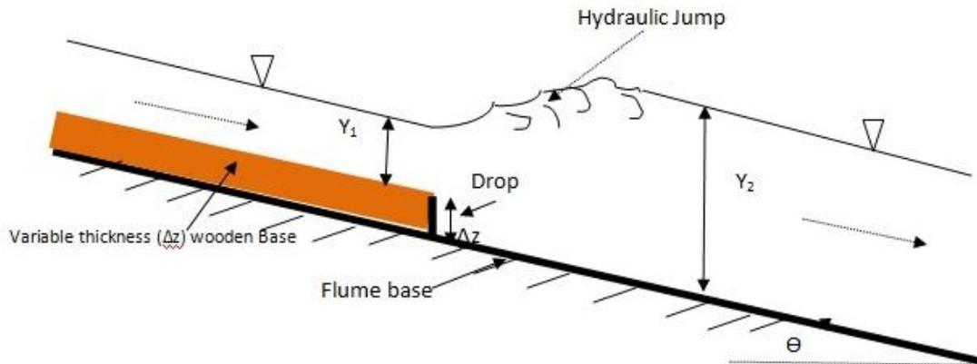
Fig. 1. Definition sketch of a hydraulic jump in a sloping channel with abrupt drop.
