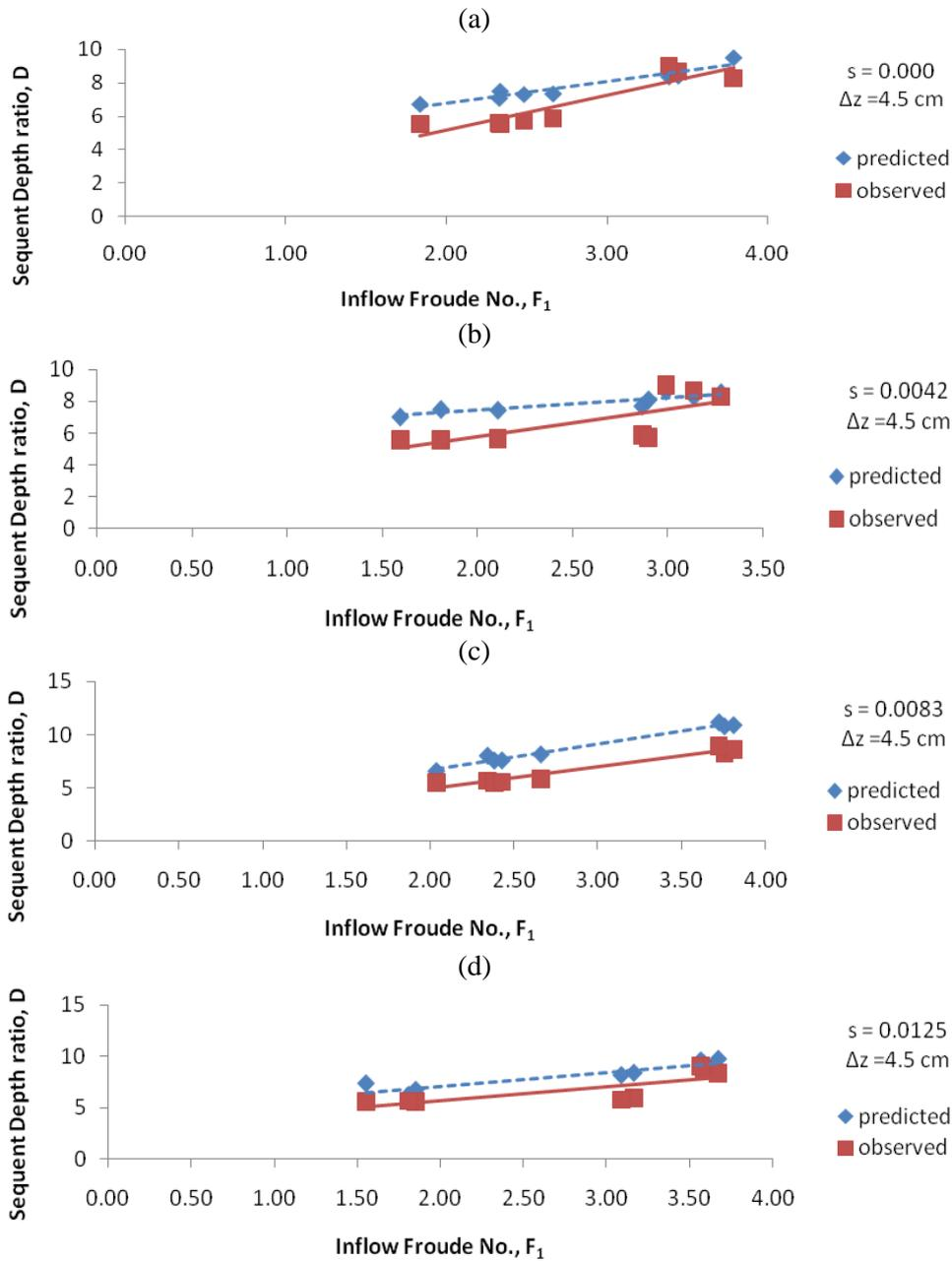
Fig. 9. D Vs  $F_1$  with drop height,  $\Delta z = 4.5$  cm; (a) Slope = 0.000 (b) Slope = 0.0042 (c) Slope = 0.0083 (d) Slope = 0.0125
