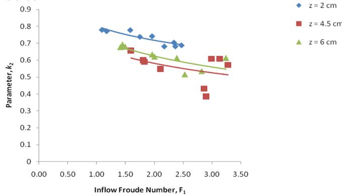
Fig. 6. Variation of parameter  $k_2$  with  $F_1$  for different drop height with Slope = 0.0042
