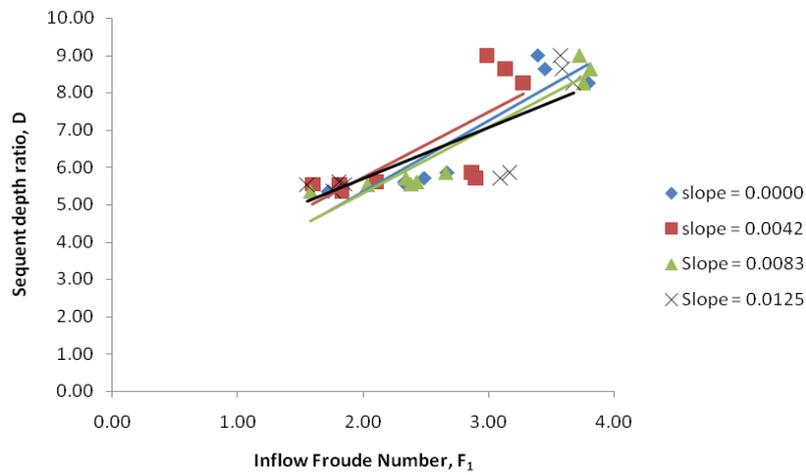
Fig. 3. D vs.  $F_1$  for different channel slopes with drop height,  $\Delta z = 4.5$  cm
