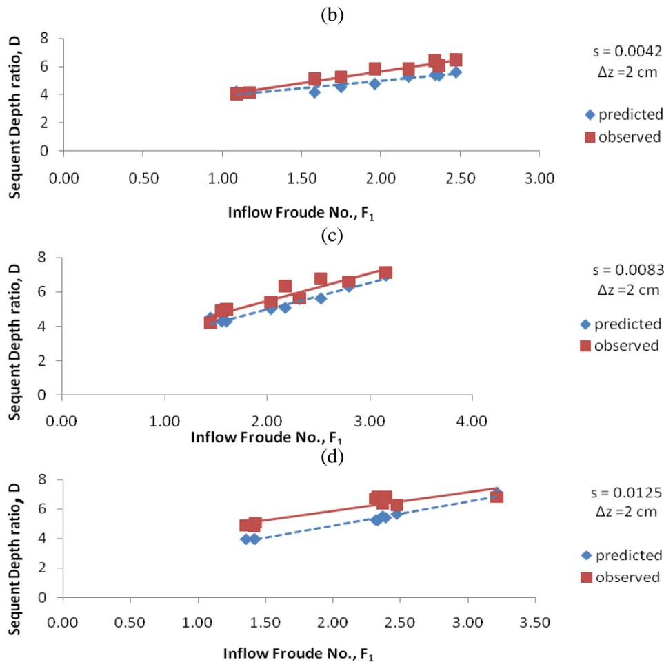
Fig. 10. D vs.  $F_1$  with drop height,  $\Delta z = 2 \text{ cm}$ ;
