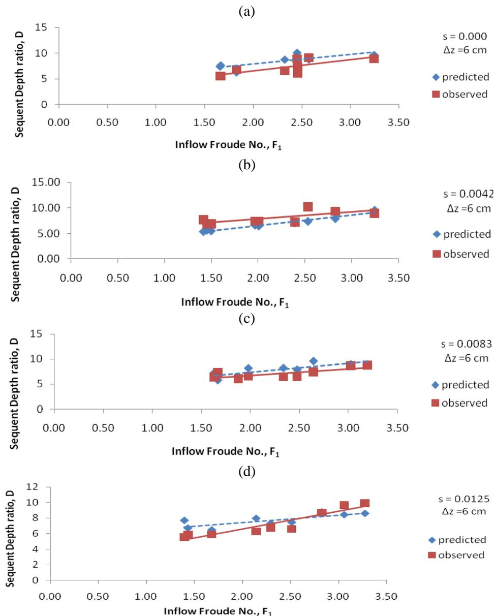
Fig. 8.  $D$  Vs  $F_1$  with drop height,  $\Delta z = 6$  cm;
