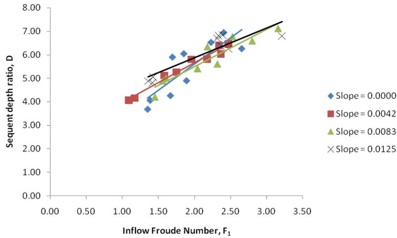
Fig. 2. D vs.  $F_1$  for different channel slopes with drop height,  $\Delta z = 2$  cm.
