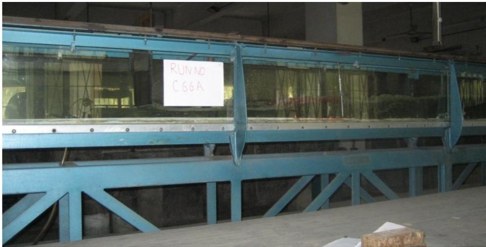
Plate 1: Photograph of the 12.2 m (40-ft) long Laboratory tilting flume
