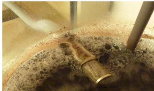
Fig. 4. Meteor Pilot Effluent pipe with Media Retaining Screen Unit & Flow Diagram.
