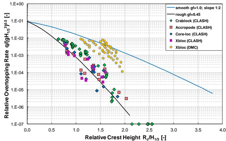
Fig. 11. Test results of crablock compare to empirical prediction and other monolayer units (using  $H_{1/3}$ )
