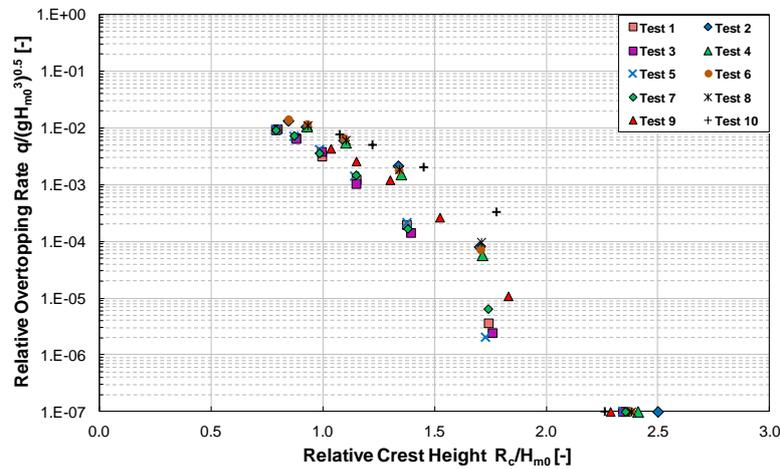
Fig. 7. Relative overtopping discharge as a function of relative freeboard
