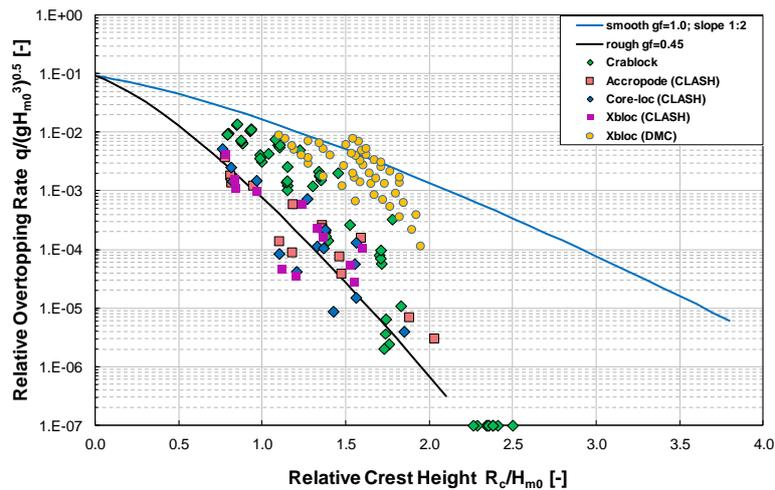
Fig. 8. Test results of crablock compare to empirical prediction and other monolayer units
