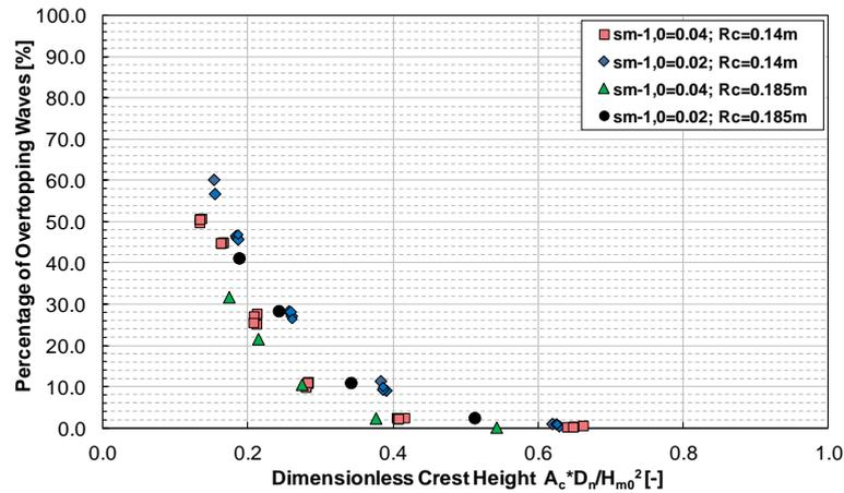
Fig. 9. Percentage of wave overtopping as a function of dimensionless crest freeboard
