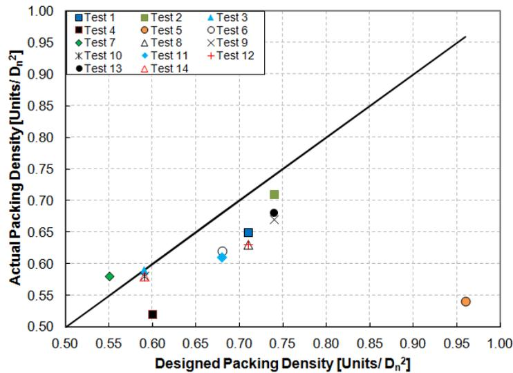
Fig. 6. Designed nominal packing density against measured nominal packing density
