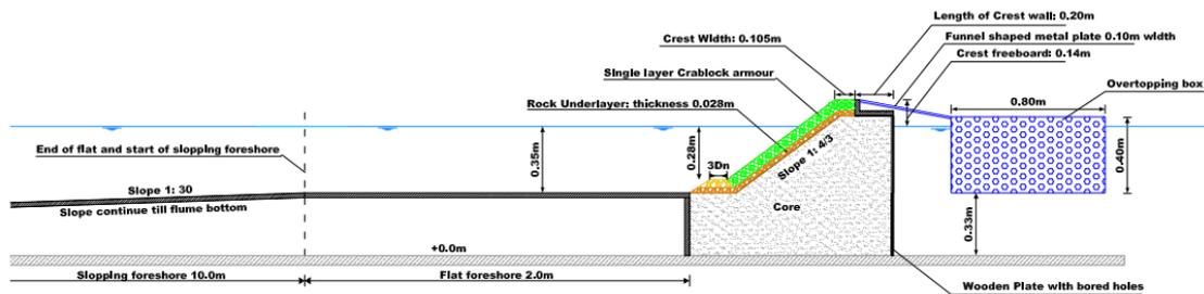
Fig. 4. Cross-section of model breakwater ( $R_c = 1.2 \times$  Design wave height); tests 1-8
