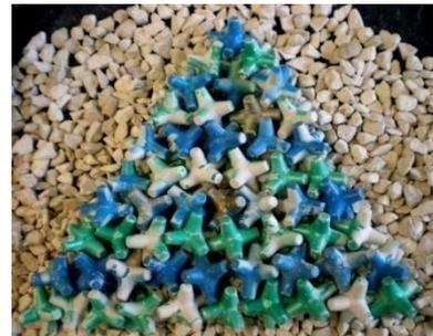
Random placement using conventional under layer in a diamond-shaped grid
