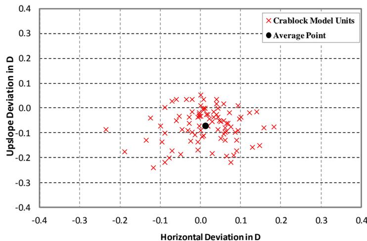
Fig. 5. Deviation of units from its intended position (Test 13)
