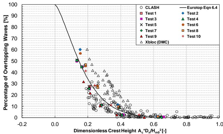
Fig. 10. Test results on percentage of overtopping compare to empirical prediction and other single layer units
