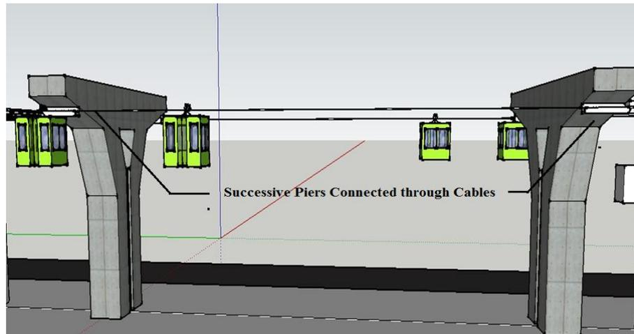
Fig. 9. Supporting pier as tower of the system.
