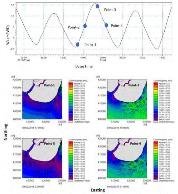
Fig. 3.2. Current direction and speed at Kuakata nearshore in dry period at different water level condition.
