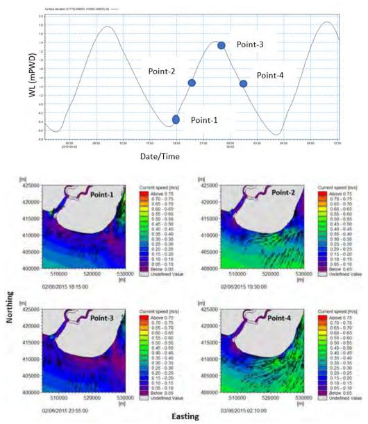
Fig. 3.1. Current direction and speed at Kuakata nearshore in monsoon period at different water level condition.
