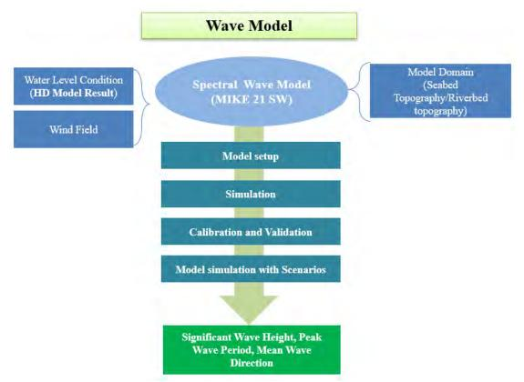
Fig. 2.13. Flow chart of wave model using MIKE 21 SW.
