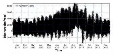
Fig. 2.3. Upstream boundary of hydrodynamic model (Hilisha river).
