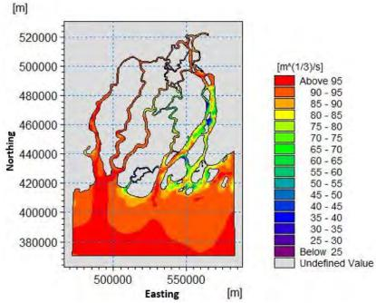
Fig. 2.6. Spatially varied manning M map used for model calibration.
