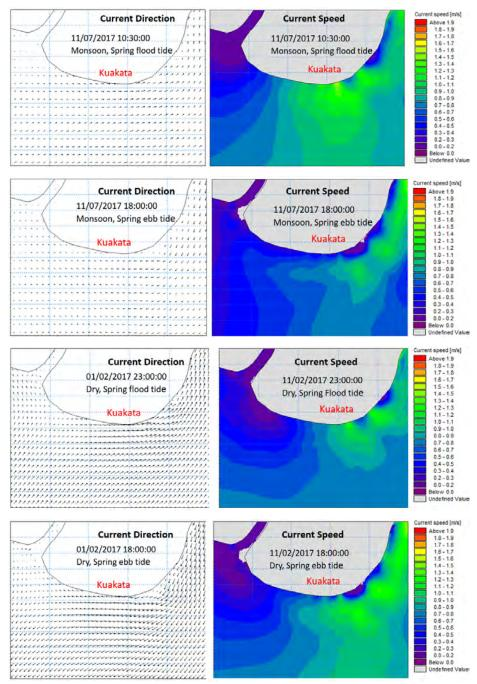
Fig. 3.5. Current speed diagram with wave action at spring tide.
