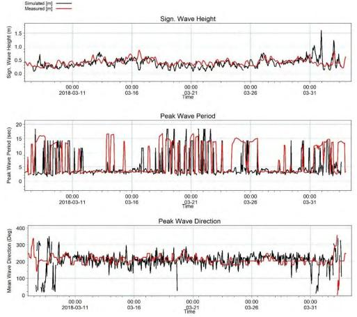
Fig. 2.16. Calibration plot of significant wave height, peak wave period and peak wave direction.
