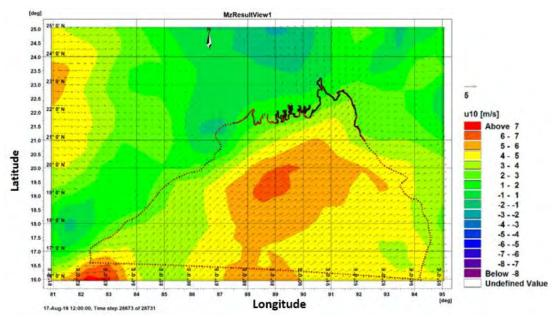
Fig. 2.15. Y-component of wind speed at a particular time covering the Bay of Bengal model area.
