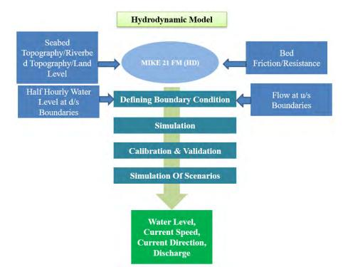
Fig. 2.1. Flow chart of a hydrodynamic model.
