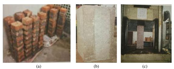
Fig. 1. (a) Brick masonry column (b) strengthened brick masonry column and (c) experimental setup.
