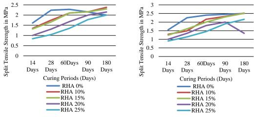
Fig. 3.4. Split tensile strength of different RHA concretes in plain water.
