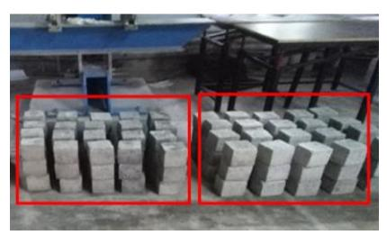
Fig. 3.1. From left, specimens exposed to sodium chloride environment and specimens exposed to plain water.
