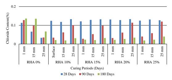
Fig. 3.6. Chloride content (%) at different depth levels of RHA concretes in NaCl environment.
