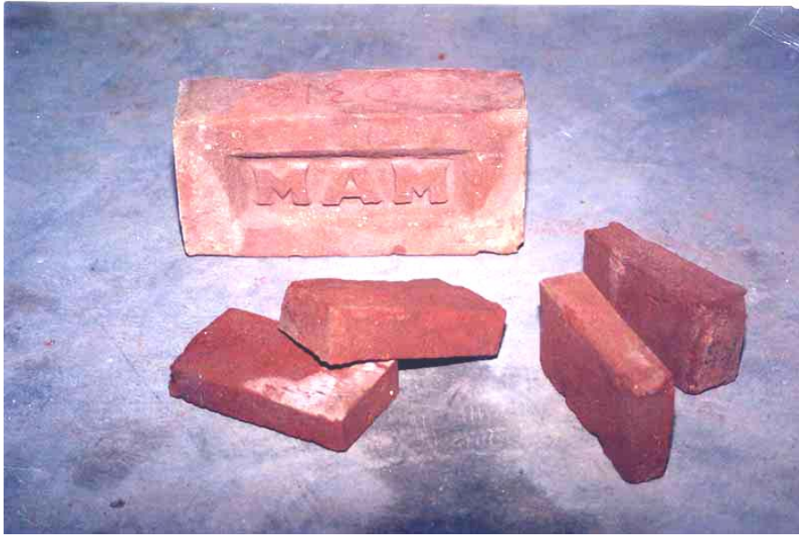
Fig. 4. Scaled down brick specimens sliced out from full sized brick
