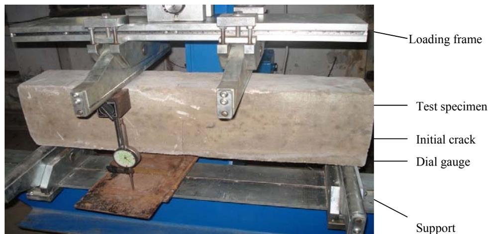
Figure 1. Experimental setup for fracture toughness test of beam specimen.
