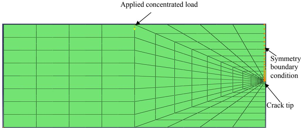
Figure 7. Finite element model of half specimen
