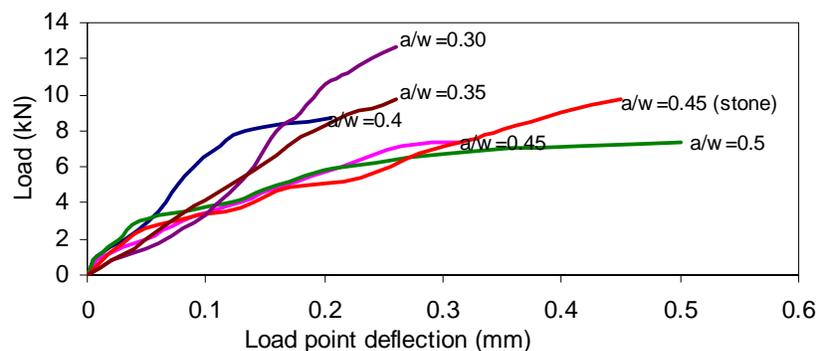
Fig. 2: Typical load-deflection plots up to peak load for various  $a/W$  ratios.
