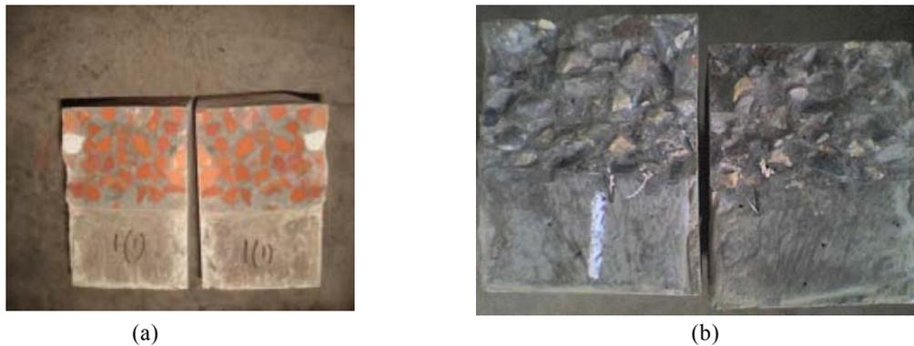
Fig. 5: Failure surfaces of tested beam made with; (a) Locally available brick aggregates and (b) Stone aggregates
