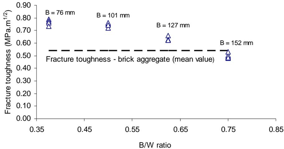
Fig. 6. Fracture toughness for various width – depth ( $B/W$ ) ratios of test specimen (depth of the specimen,  $W = 0.2032$  m)
