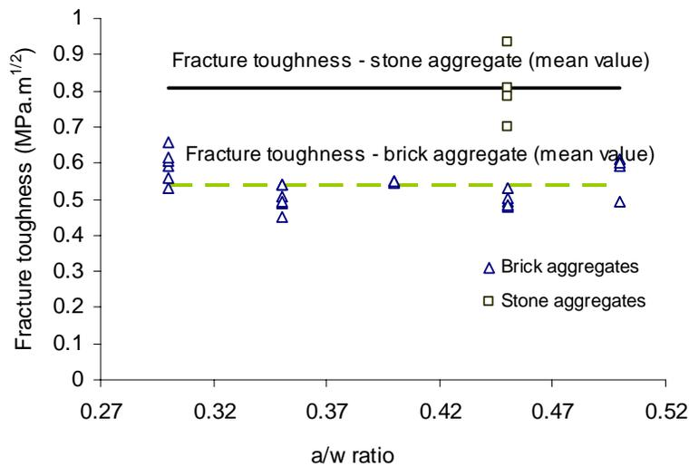
Figure 3. Fracture toughness for various  $a/W$  ratios ( $a$  = crack depth,  $W$  = depth of the specimen = 0.2032 m)
