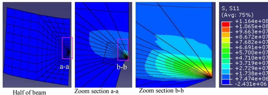
Figure 8. Stress contour plot for stress in local 1-direction around the crack tip
