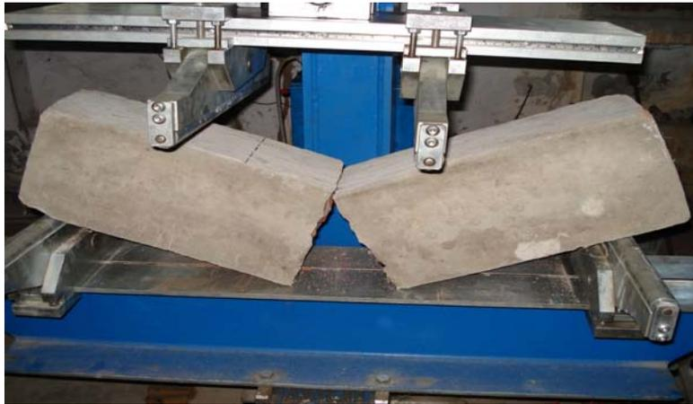
Fig. 4: Direction of crack propagation in the specimen made with industry-burnt brick aggregates from the pre-existing crack
