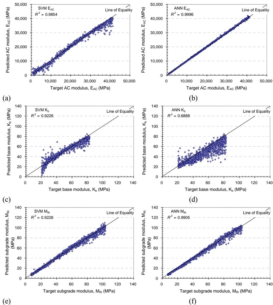
Figure 5. Targeted vs. predicted pavement layer modulus values.
