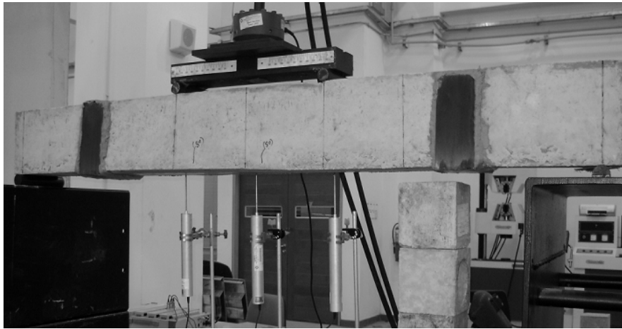
Figure 5. Typical four-point bending test set up
