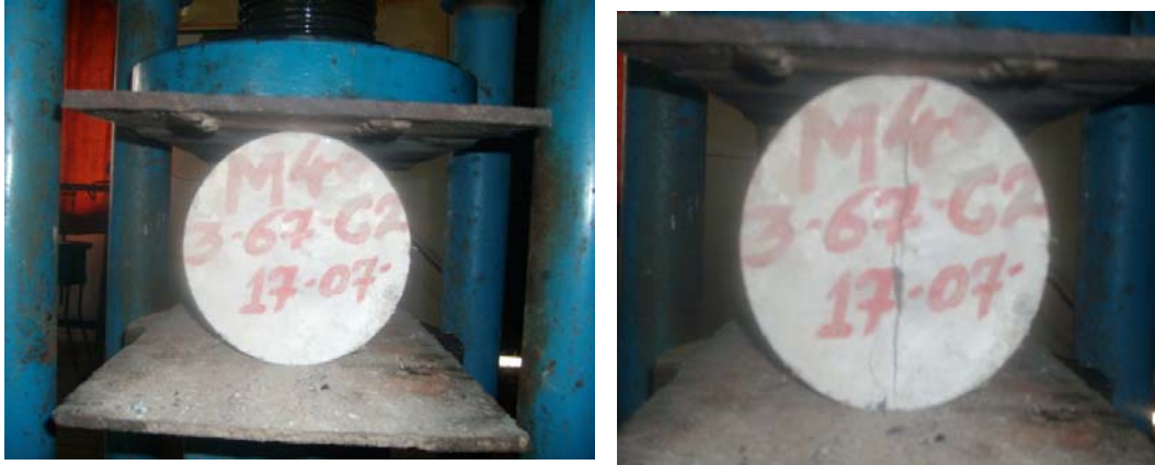
Fig. 1. Testing of tensile strength test specimen
