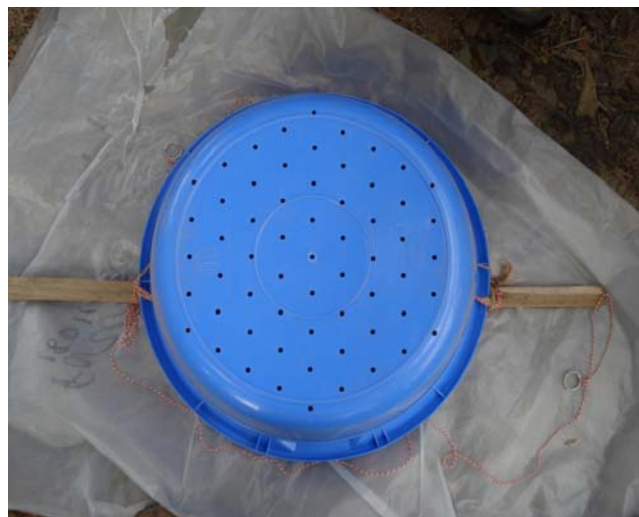
Figure 6: Sand discharge bowl with 4 mm diameter holes.
