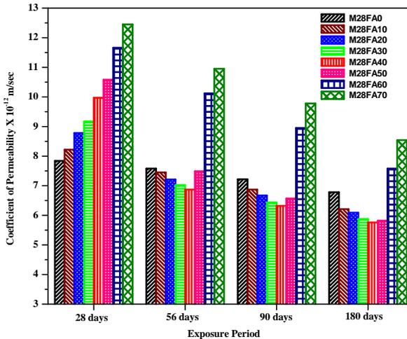
Fig.9 : Permeability - Exposure Time Relation for M28 Fly Ash Concretes
