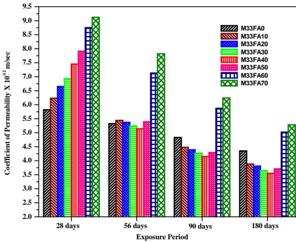
Fig.8 : Permeability - Exposure Time Relation for M33 Fly Ash Concretes
