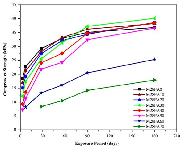
Fig.3 : Compressive Strength - Exposure Time Relation for M28 Fly Ash Concretes
