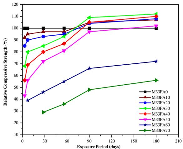
Fig.5 : Relative Compressive Strength - Exposure Time Relation for M33 Fly Ash Concretes
