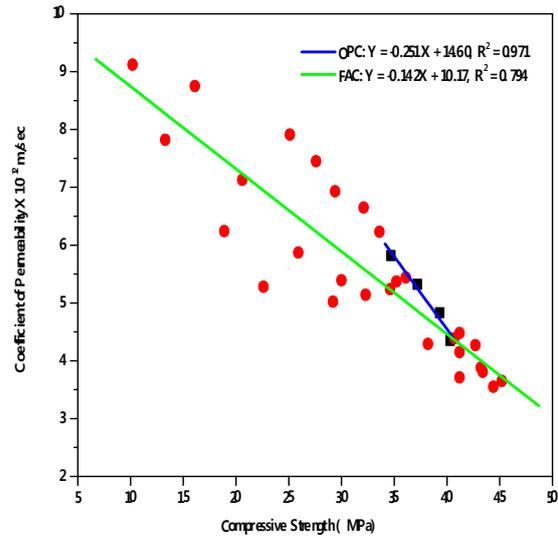
Fig.14: Permeability - Compressive Strength Relation for OPC and FAC Concretes of Grade M35
