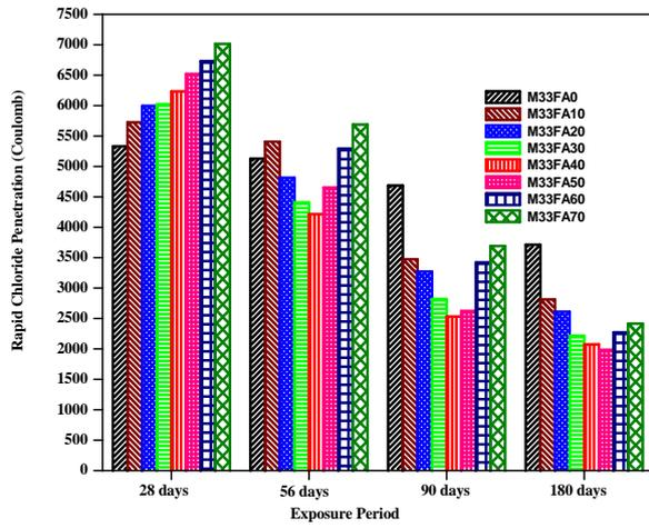
Fig.11 : Rapid Chloride Penetration - Exposure Time Relation for M33 Fly Ash Concretes
