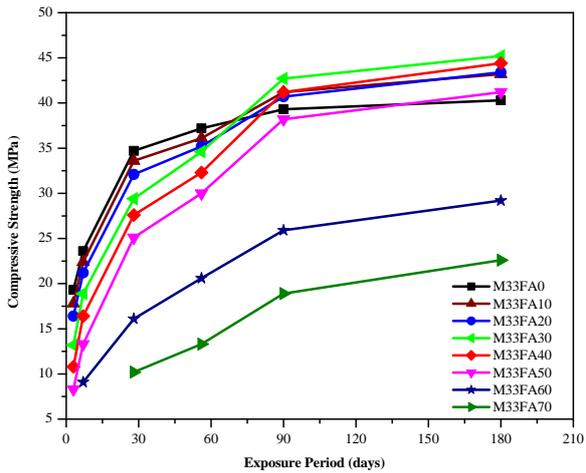
Fig.2 : Compressive Strength - Exposure Time Relation for M33 Fly Ash Concretes
