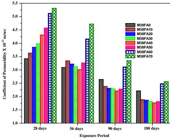
Fig.7 : Permeability - Exposure Time Relation for M38 Fly Ash Concretes
