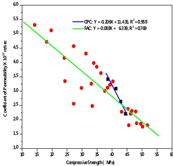
Fig.13: Permeability - Compressive Strength Relation for OPC and FA Concretes of Grade M38
