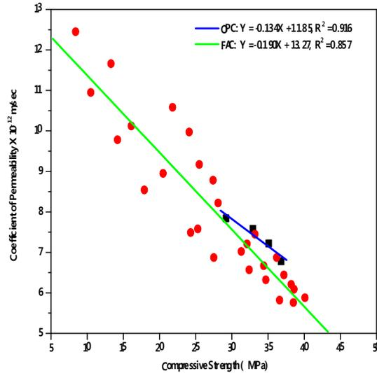
Fig.15: Permeability - Compressive Strength Relation for OPC and FAC Concretes of Grade M30
