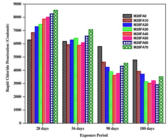
Fig.12 : Rapid Chloride Penetration - Exposure Time Relation for M28 Fly Ash Concretes
