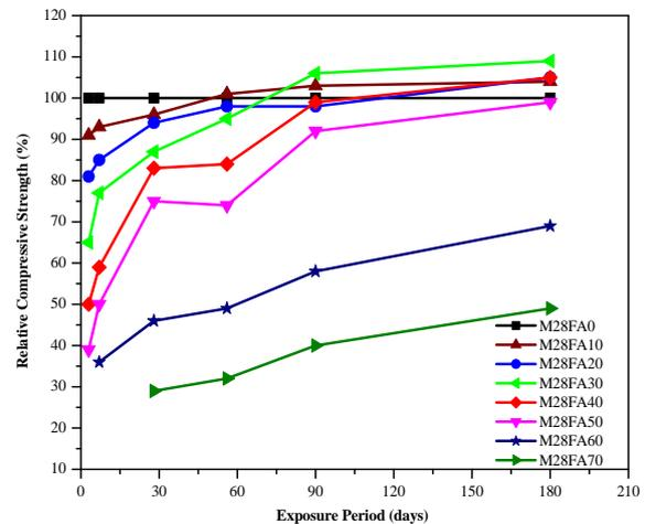
Fig.6 : Relative Compressive Strength - Exposure Time Relation for M28 Fly Ash Concretes
