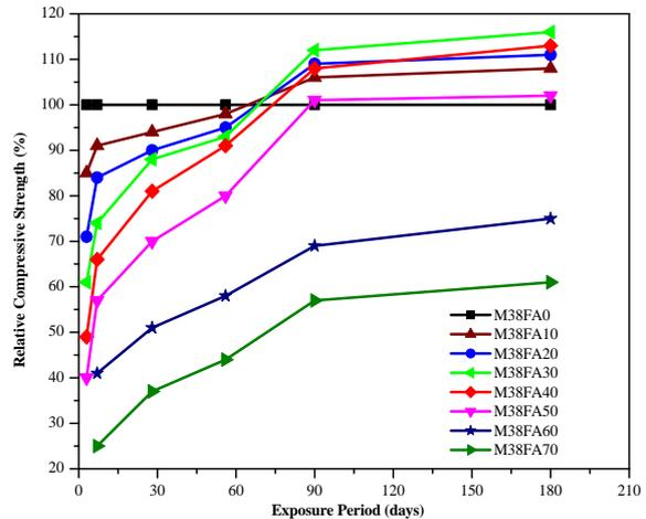
Fig.4 : Relative Compressive Strength - Exposure Time Relation for M38 Fly Ash Concretes
