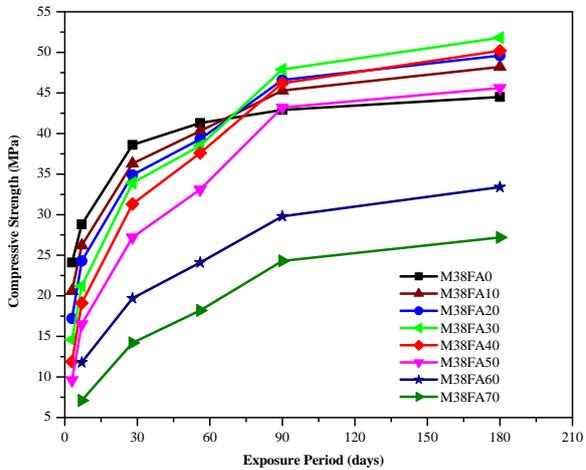
Fig.1 : Compressive Strength - Exposure Time Relation for M38 Fly Ash Concretes
