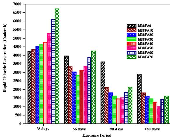
Fig.10 : Rapid Chloride Penetration - Exposure Time Relation for M38 Fly Ash Concretes
