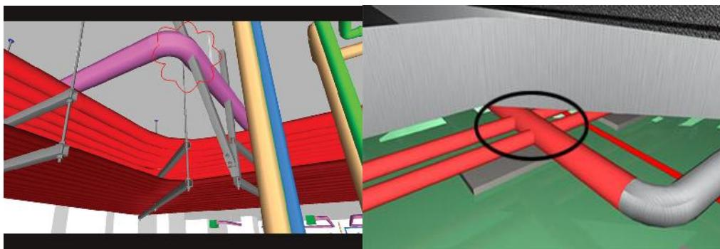
Fig. 7. Clash Detection by BIM software
