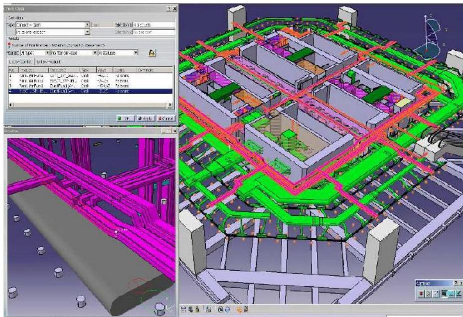
Fig. 9. Automated Clash Detection in OIE Project (Gammon Construction Ltd, HK)
