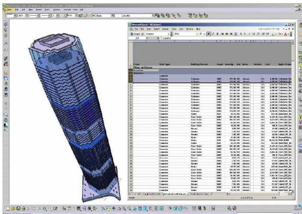
Fig. 11. Preparation of Automated Estimates (Gammon Construction Ltd, HK)
