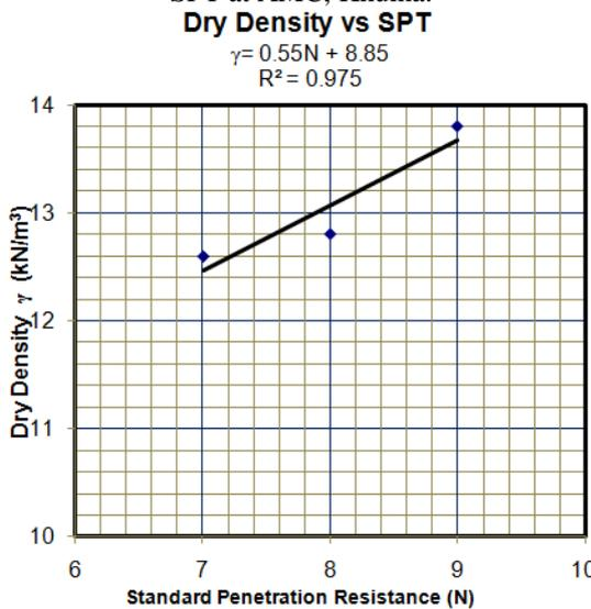
Fig. 22. Relationship between Dry Density & SPT at AMC, Khulna.
