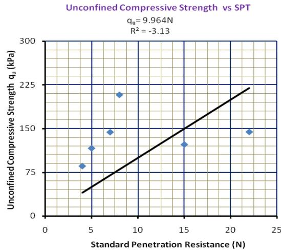
Fig. 14. Correlation between Unconfined Compressive Strength ( $q_u$ ) & Standard Penetration Resistance (N) (for  $LL \geq 50$ )
