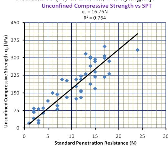
Fig. 8. Combined Correlation between unconfined Compressive Strength ( $q_u$ ) & Penetration Resistance (N) at Dhaka Cantonment and Bhulta Narayanganj.
