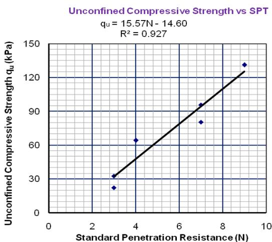
Fig. 10. Correlation between Unconfined Compressive Strength ( $q_u$ ) & Penetration Resistance (N) at AMC, Khulna.
