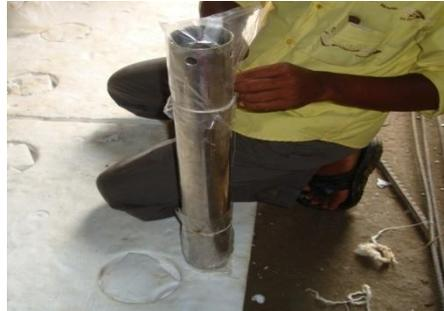
Fig. 5. Covering after waxing to make the sample airtight.
