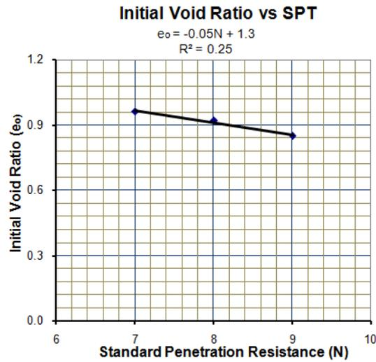
Fig. 20. Relationship between Initial Void ratio & SPT at AMC, Khulna.
