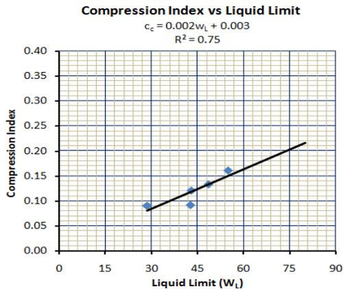
Fig. 23. Correlation between Compression Index & Liquid Limit at Bhulta, Narayanganj.
