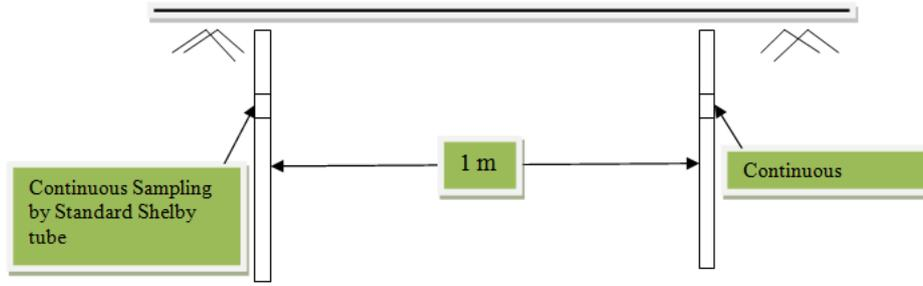
Fig. 4. Schematic diagram of boreholes arranged in the field.
