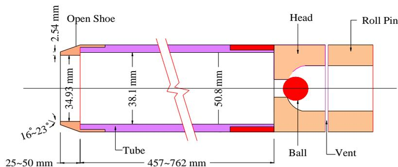
Fig. 1. Standard Dimension of SPT Split-Barrel Sampler (ASTM D 1586-08a).
