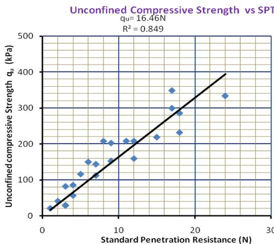
Fig. 12. Summary of combined Relationship between SPT (N) & Unconfined Compressive Strength ( $q_u$ ) at Khulna, Narayanganj and Dhaka.
