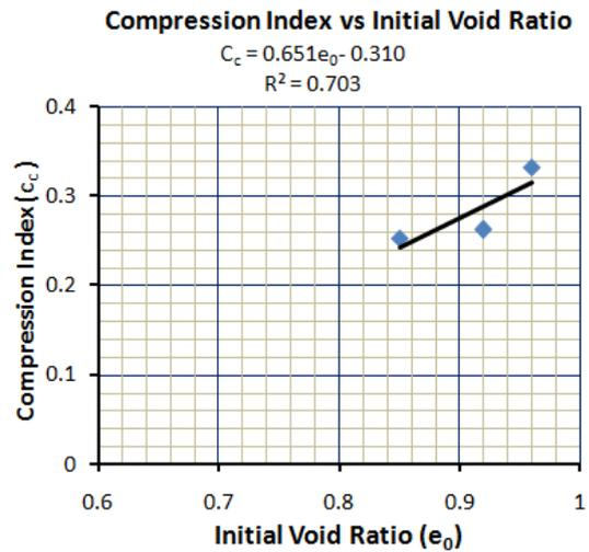
Fig. 28. Correlation between Compression Index & Initial Void Ratio at AMC, Khulna.
