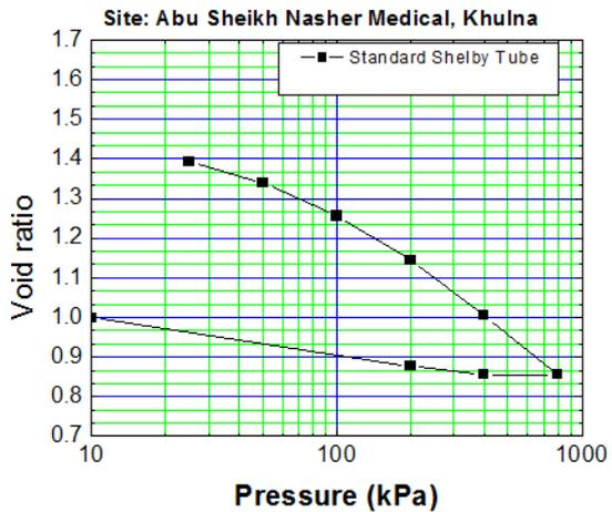
Fig. 16. Typical e-log p curve of samples collected from SANH site, Khulna.
