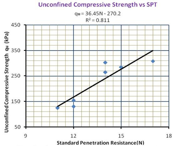
Fig. 7. Correlation between unconfined Compressive Strength ( $q_u$ ) & Penetration Resistance (N) at Dhaka Cantonment.
