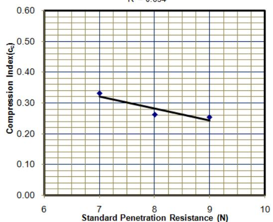
Fig. 18. Relationship between SPT & Compression Index at AMC, Khulna.
