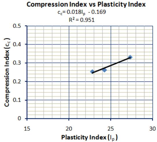
Fig. 26. Correlation between Compression Index & Plasticity Index at AMC, Khulna.
