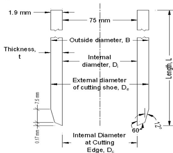
Fig. 3. Schematic diagram of Standard Shelby tube.
