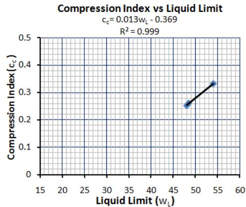
Fig. 24. Correlation between Compression Index & Liquid Limit at AMC, Khulna.
