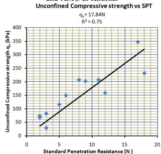
Fig. 13. Correlation between Unconfined Compressive Strength ( $q_u$ ) & Standard Penetration Resistance (N) (for  $LL \leq 50$ )
