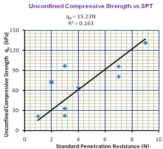
Fig. 11. Combined Correlation between Unconfined Compressive Strength ( $q_u$ ) & Standard Penetration Resistance (N) at SANH and AMC at Khulna.
