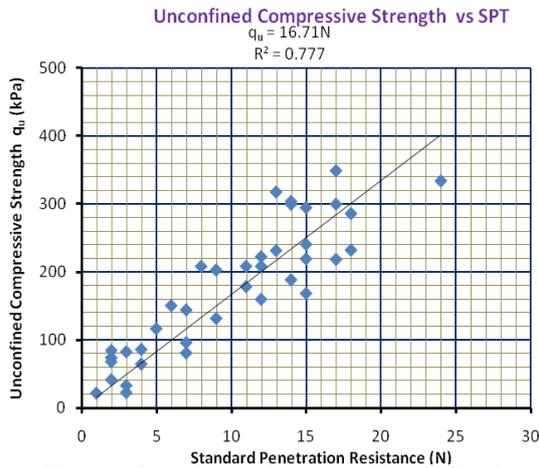
Fig. 6. Correlation between Unconfined Compressive Strength ( $q_u$ ) & Penetration Resistance (N) at Bhulta, Narayanganj.
