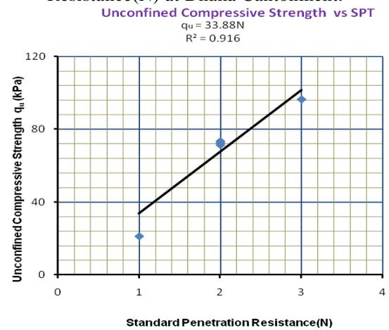
Fig. 9. Correlation between unconfined Compressive Strength ( $q_u$ ) & Penetration Resistance (N) at SANH, Khulna.
