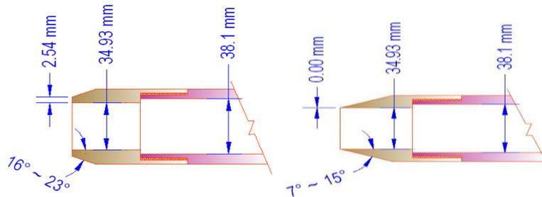
Fig. 2. Comparison of dimension between Standard shoe and Conventional Shoe of SPT spoon.
