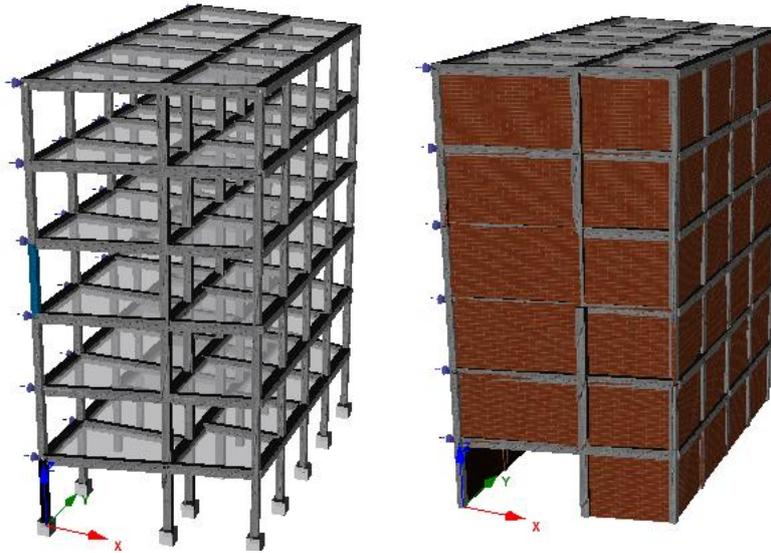
Fig. 5. (a) Bare frame model; (b) Frame with Infill walls model.
