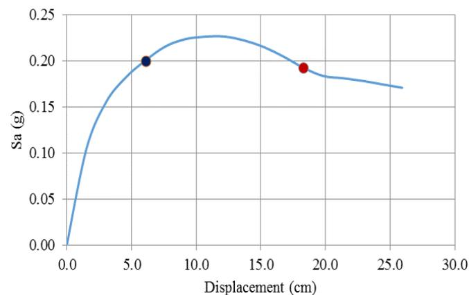
Fig. 11. Capacity curve for Infill model.
