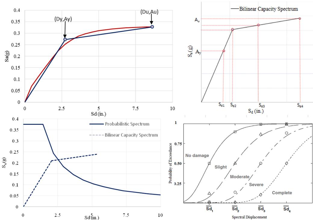
Fig. 6. a) An example of capacity curve and its simplified bilinear form; b) damage state definition; c) capacity spectrum performance and d) fragility curves for damage states.
