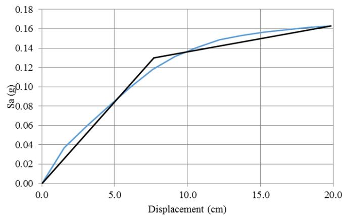
Fig. 10. Capacity curve of bare frame model
