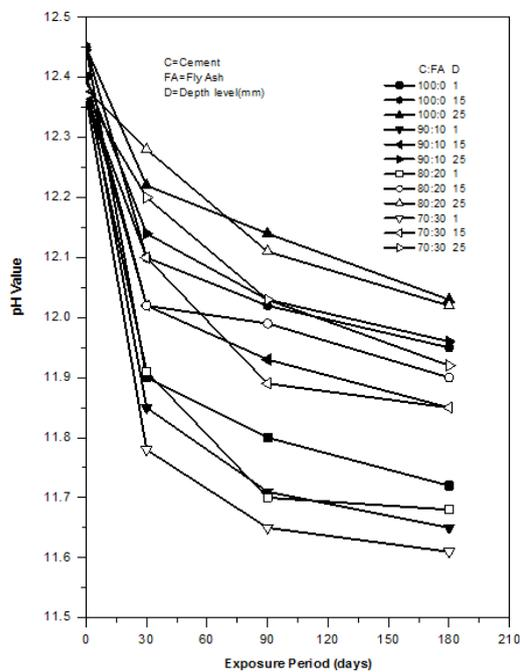
Fig. 10. pH value – exposure time relation for fly ash concretes exposed to sea water of 5T concentration.
