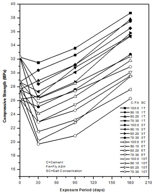
Fig. 4. Compressive strength-exposure time relation for fly ash concretes exposed to different marine environments.
