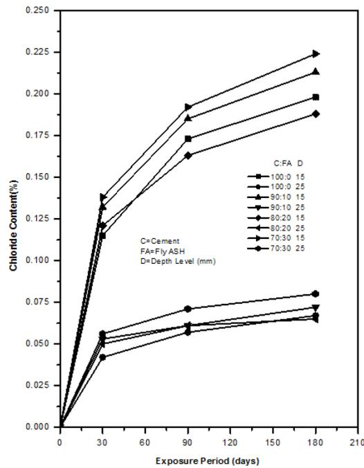
Fig. 7. Chloride content-exposure time relation for fly ash concretes exposed to sea water of 5T concentration.
