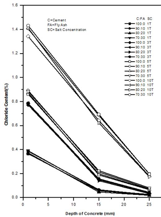
Fig. 9. Chloride concentration profile for fly ash concretes exposed to different marine environments (Age 6 months).
