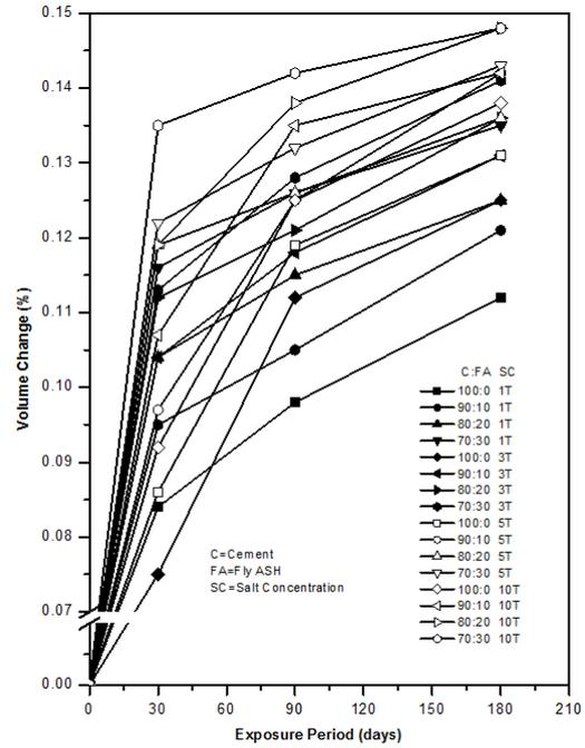
Fig. 3. Volume change-exposure time relation for fly ash concretes exposed to different marine environments.
