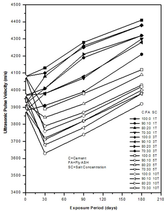
Fig. 6. UPV-exposure time relation for fly ash concretes exposed to different marine Environments.
