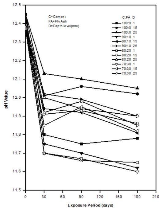
Fig. 11. pH value – exposure time relation for fly ash concretes exposed to sea water of 10T concentration.
