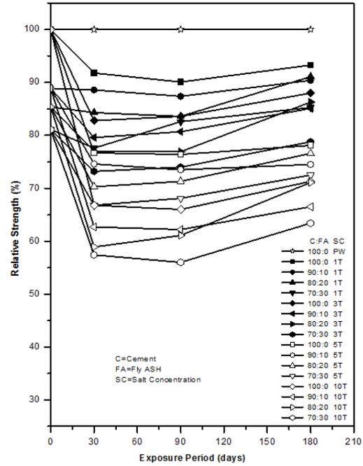
Fig. 5. Relative strength-exposure time relation for fly ash concretes exposed to different marine environments.
