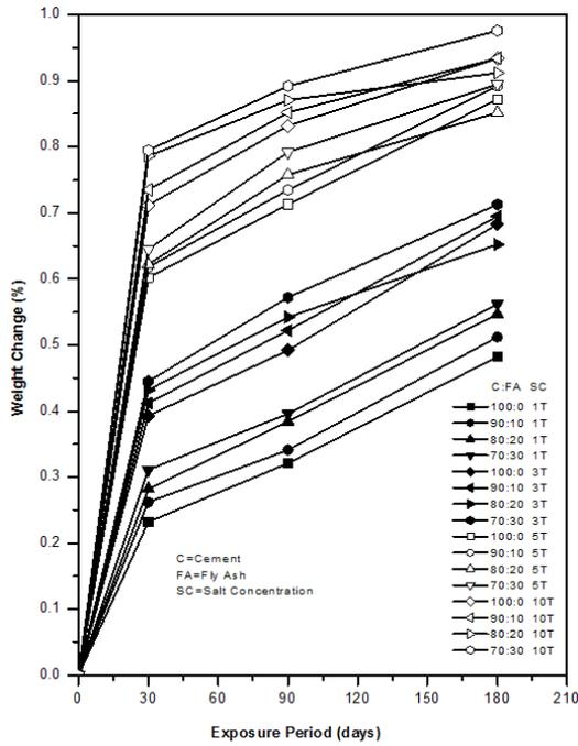
Fig. 2. Weight change-exposure time relation for fly ash concretes exposed to different marine environments.
