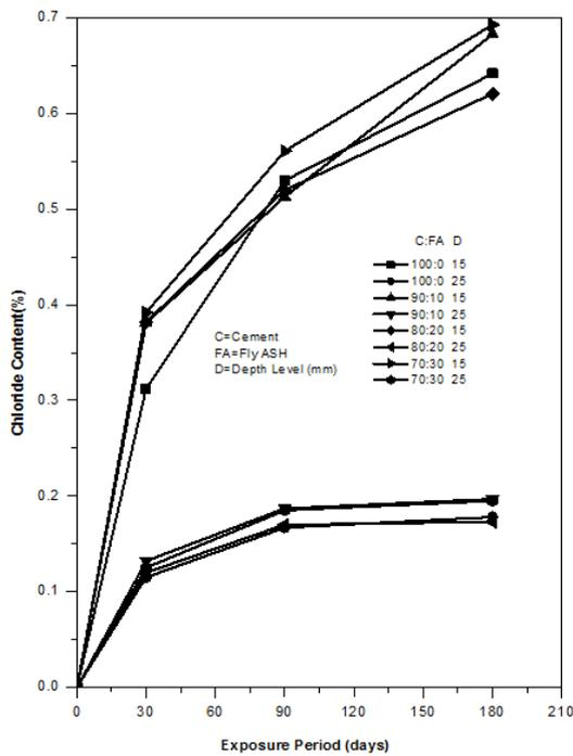
Fig. 8. Chloride content-exposure time relation for fly ash concretes exposed to sea water of 10T concentration.
