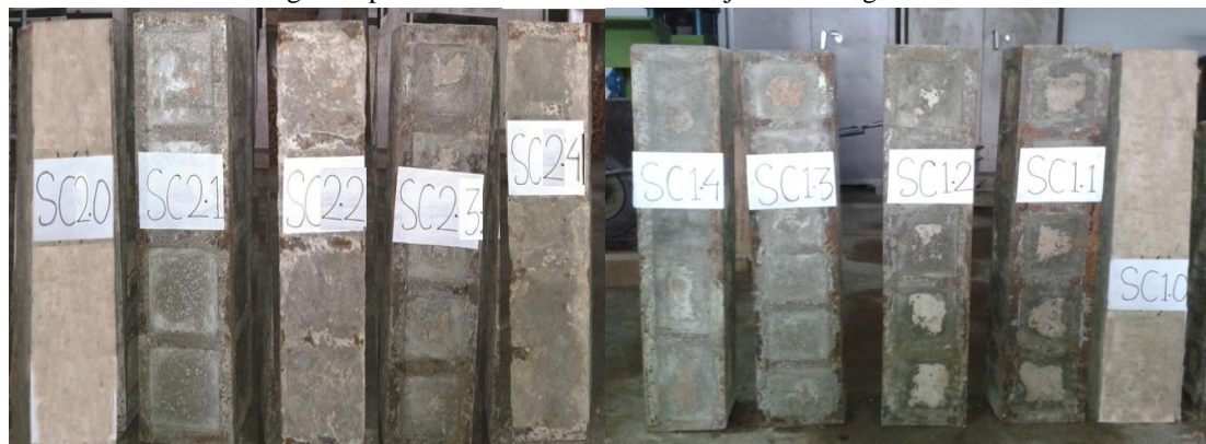
Fig. 2. Strengthened specimens after casting and jacket erection.
