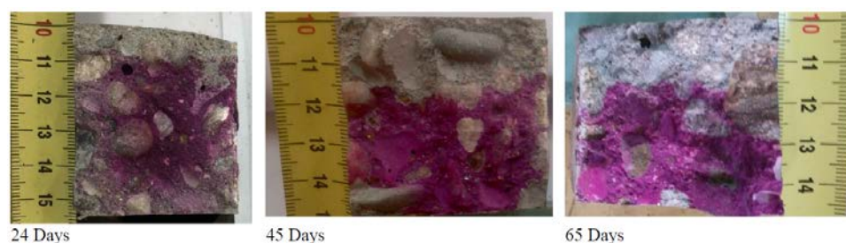
Fig. 23. Carbonation of concrete at different ages for round shaped stone (CEM Type II B M, W/C = 0.45, C = 400 kg/m 3 ).
