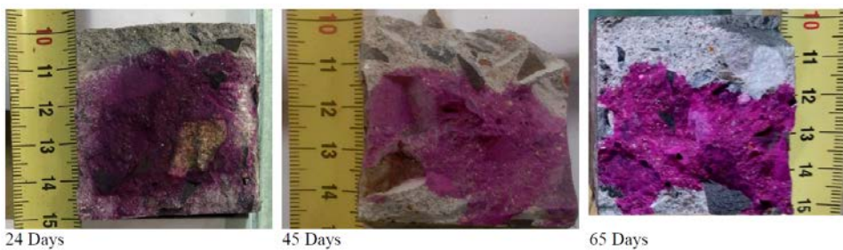
Fig. 22. Carbonation of concrete at different ages for black stone chips (CEM Type II B M, W/C = 0.45, C = 400 kg/m 3 ).
