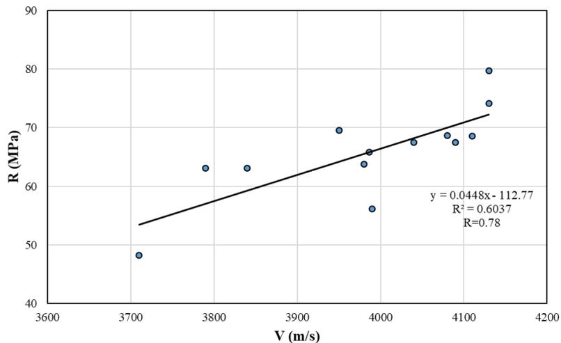
Fig. 11. Calibration dependence graph between ultrasonic test & pull-out test results.
