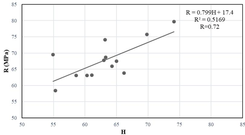
Fig. 10. Calibration dependence graph between shock pulse test & pull-out test results.
