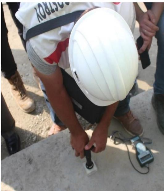
Fig. 2(a). Checking the shock impulse machine using reference prism.
