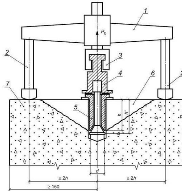
1 - device with a loading device and a load cell; 2 - support loading device; 3 - gripping the loading device; 4 - transition elements, thrust; 5 - anchor device; 6 - breakable concrete (separation cone); 7 - tested design
