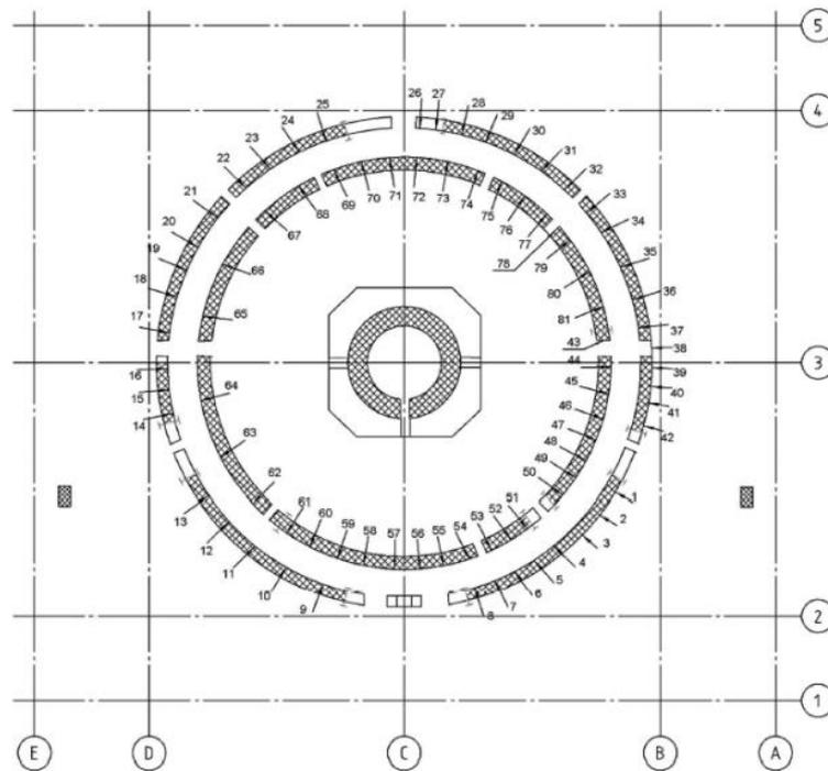
Fig. 1. Different sections of inner and outer corridor wall have been numbered for NDT.
