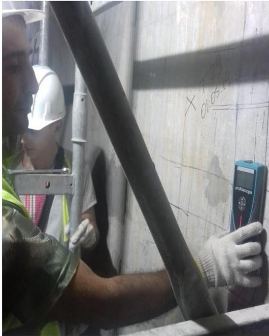
Fig. 5(a). Usage of Rebar Locator.
