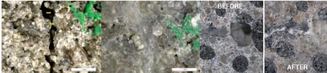
Fig. 1. Healing of a crack in mortar (average diameter 507  $\mu$ m) with *B. sphaericus* hydrogels; left: initial crack, applied at the mortar age of 28d; right: healed crack after four weeks incubation in wet-dry cycles of 1 h water submersion and 11 h at 60 percent RH (From Wang et. al 2014)).
