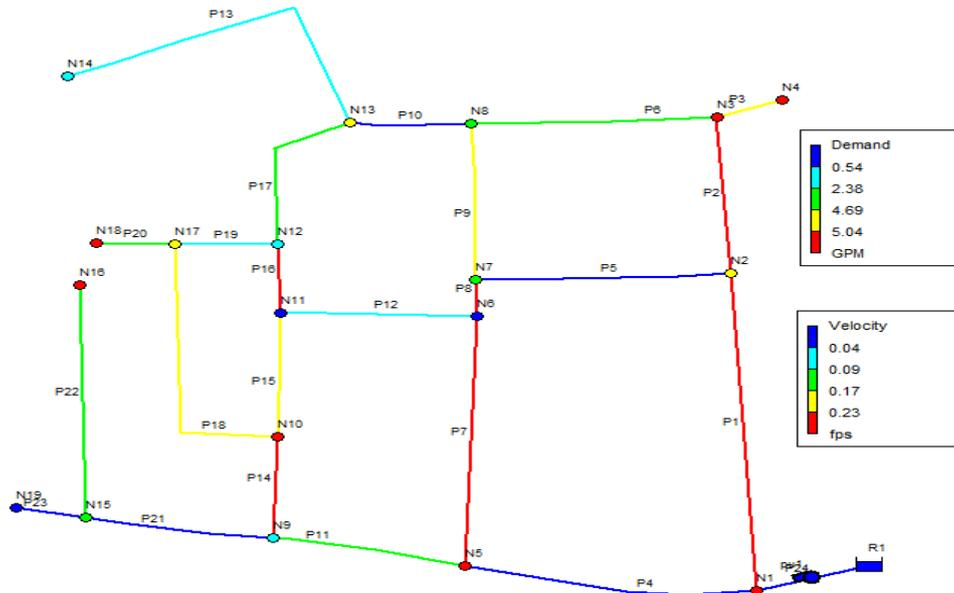
Fig. 12(a). Simulated demand and velocity for the study area during leaks at 8 am.
