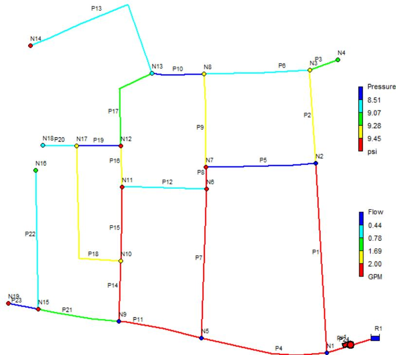
Fig. 3. Illustration of predicted pressure and flows using the EPANET graphical interface.
