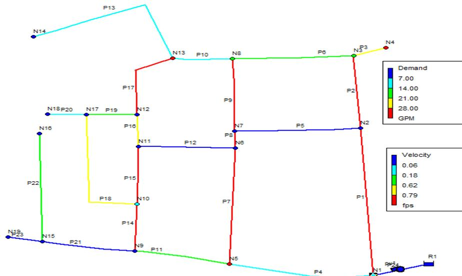
Fig. 12(b). Simulated demand and velocity for the study area during leaks at 8 am.
