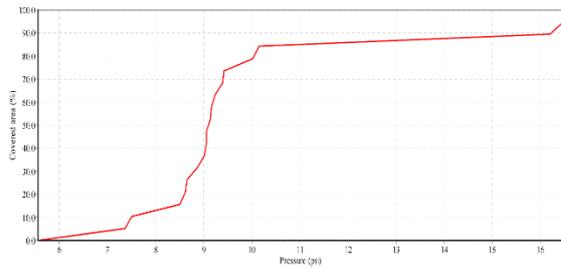
Fig. 4. Numerical distribution of pressure in sub-system (peak hours).
