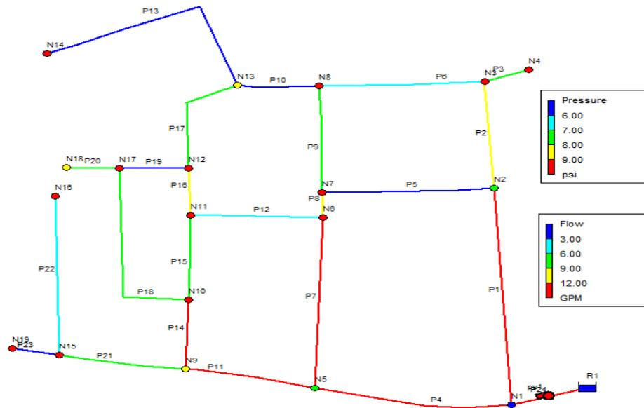
Fig. 11(a). Simulated pressure and flow for the study area during leaks at 8am.
