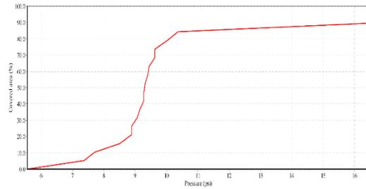
Fig. 5. Numerical distribution of pressure in sub-system (off-peak hours).
