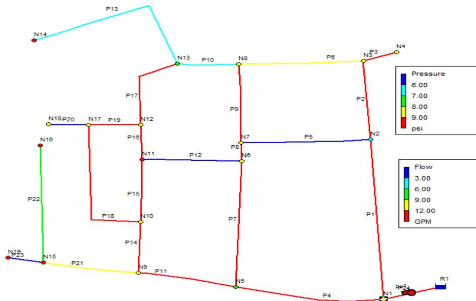
Fig. 11(b). Simulated pressure and flow for the study area after repairing at 8 am.
