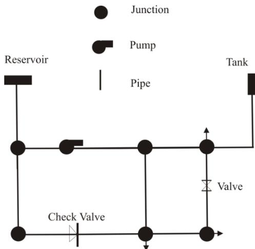
Fig. 1. Node-link representation of a water distribution network.
