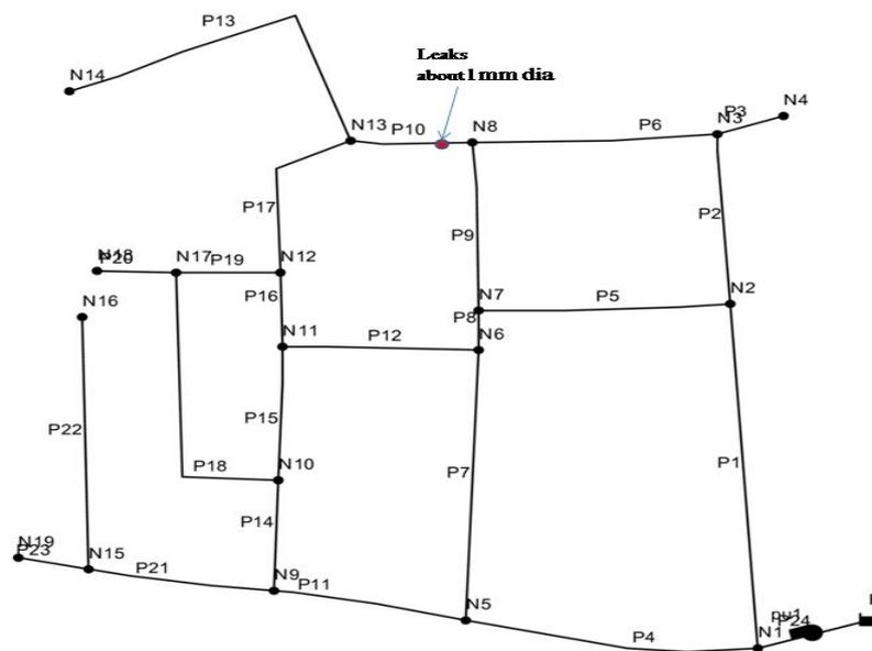
Fig. 10. EPANET network showing two leaks location in service line.
