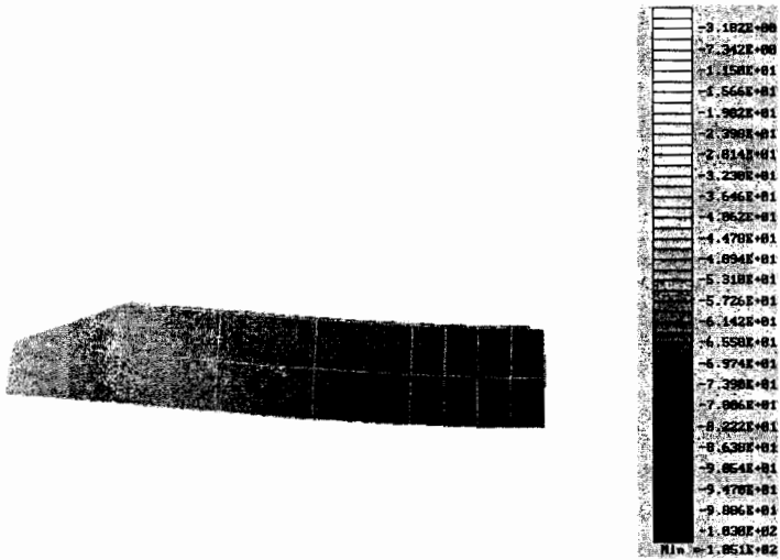
Fig 7. Contour of vertical deformation for W10
